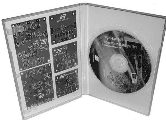
Figure 22: Evaluation kit for high speed op-amps
