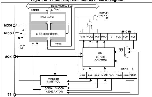
Figure 42. Serial peripheral interface block diagram
