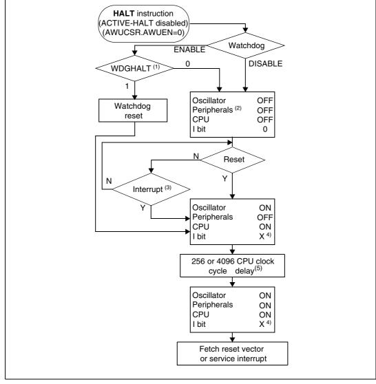
Figure 25. HALT mode flowchart
