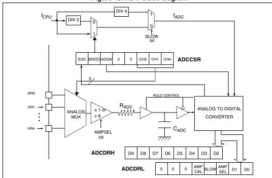
Figure 49. ADC block diagram
