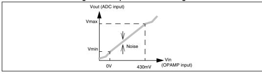
Figure 92. Amplifier noise vs voltage
