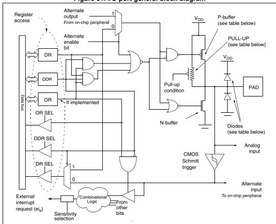
Figure 31. I/O port general block diagram
