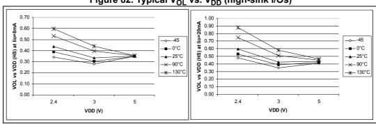
Figure 82. Typical V<sub>OL</sub> vs. V<sub>DD</sub> (high-sink I/Os)
