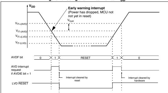
Figure 19. Using the AVD to monitor V<sub>DD</sub>
