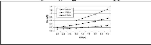
Figure 64. Typical  $I_{DD}$  in AWUF mode at  $T_A$  = 25°C
