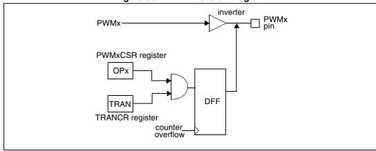
Figure 35. PWM inversion diagram
