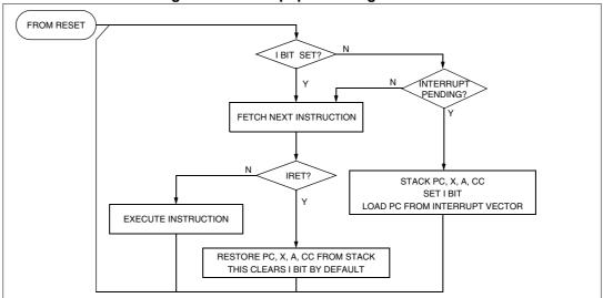
Figure 20. Interrupt processing flowchart
