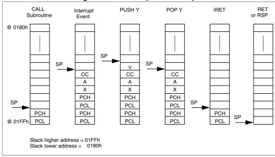
Figure 11. Stack manipulation example
