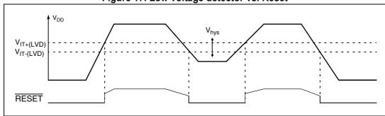
Figure 17. Low voltage detector vs. Reset
