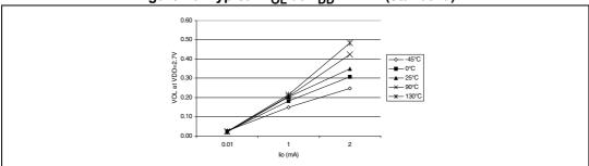
Figure 71. Typical  $V_{OL}$  at  $V_{DD}$  = 3.3V (standard)
