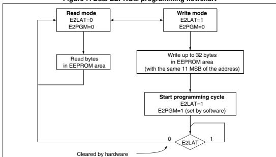
Figure 7. Data EEPROM programming flowchart
