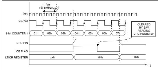
Figure 41. Input capture timing diagram
