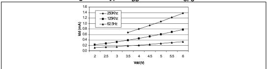
Figure 62. Typical  $I_{\rm DD}$  in WAIT vs.  $f_{\rm CPU}$
