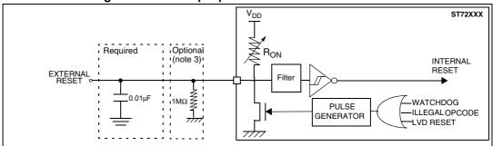
Figure 85. RESET pin protection when LVD is disabled
