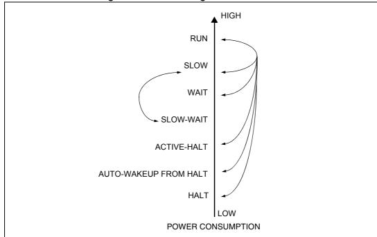
Figure 21. Power saving mode transitions
