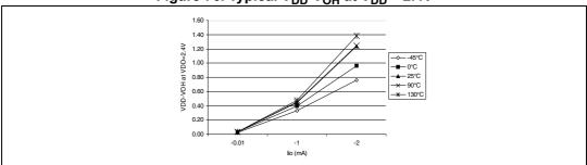
Figure 77. Typical  $V_{DD}$ - $V_{OH}$  at  $V_{DD}$  = 2.7V
