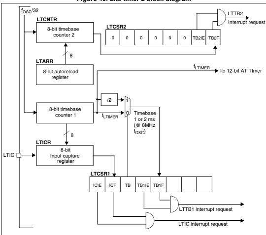
Figure 40. Lite timer 2 block diagram
