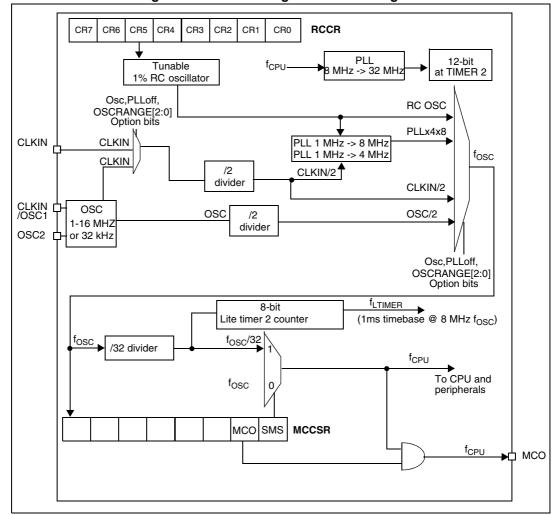
Figure 13. Clock management block diagram
