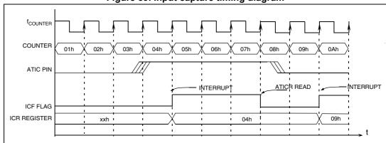
Figure 39. Input capture timing diagram
