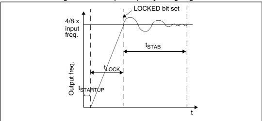
Figure 12. PLL output frequency timing diagram
