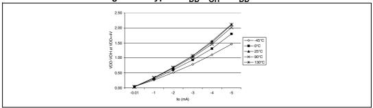
Figure 80. Typical  $V_{DD}$ - $V_{OH}$  at  $V_{DD}$  = 5V
