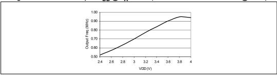
Figure 54. RC Osc Freq vs V<sub>DD</sub> (calibrated with RCCR0: 5V@ 25°C)
