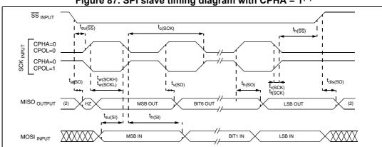
Figure 87. SPI slave timing diagram with CPHA =  $1^{(1)}$
