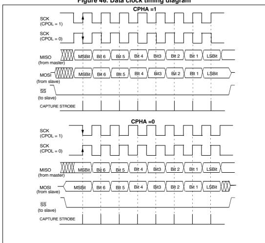
Figure 46. Data clock timing diagram
