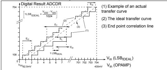
Figure 91. ADC accuracy characteristics with amplifier enabled
