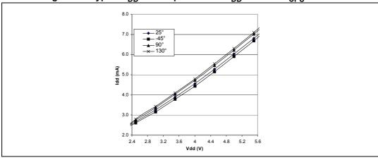
Figure 65. Typical  $I_{DD}$  vs. temperature at  $V_{DD}$  = 5V and  $f_{CPU}$  = 8MHz
