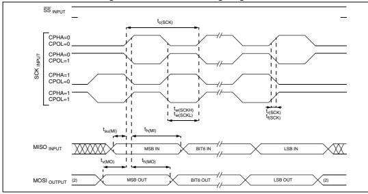
Figure 88. SPI master timing diagram<sup>(1)</sup>
