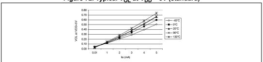
Figure 73. Typical  $V_{OL}$  at  $V_{DD}$  = 2.4V (high-sink)
