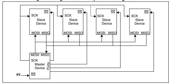
Figure 48. Single master / multiple slave configuration
