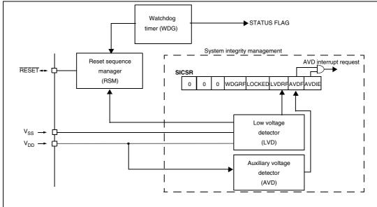
Figure 18. Reset and supply management block diagram
