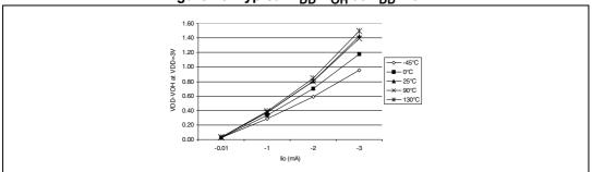
Figure 79. Typical  $V_{DD}$ - $V_{OH}$  at  $V_{DD}$  = 4V
