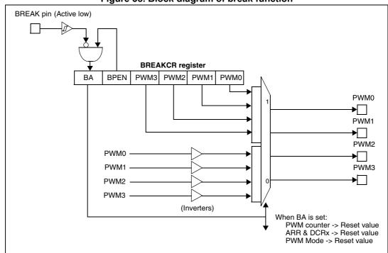
Figure 38. Block diagram of break function
