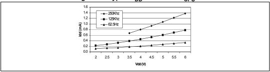
Figure 63. Typical  $I_{DD}$  in SLOW-WAIT vs.  $f_{CPU}$
