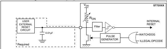
The reset network protects the device against parasitic resets.
