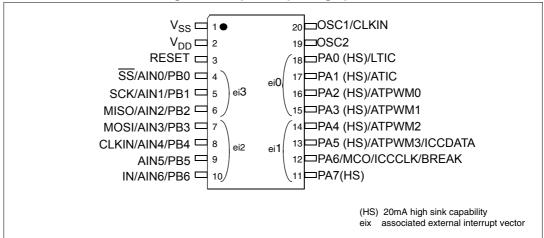
Figure 3. 20-pin DIP package pinout
