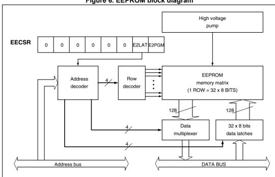
Figure 6. EEPROM block diagram
