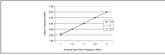
Figure 58. PLLx4 Output vs CLKIN frequency
