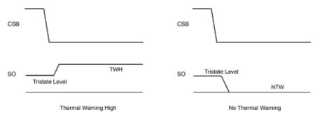
Figure 26. Accessing Thermal Warning Bit
