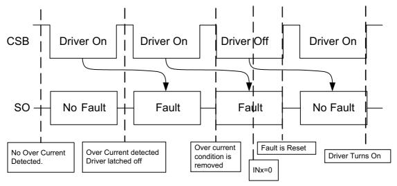
Figure 31. Over Current Timing Diagram
