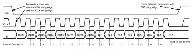
Figure 24. Frame Detection
