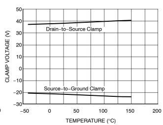
Figure 21. Output Clamp vs. Temperature
