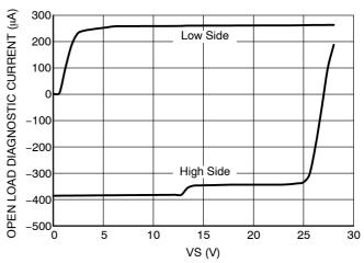
Figure 19. Open Load Detect Current vs. VS @ 25°C
