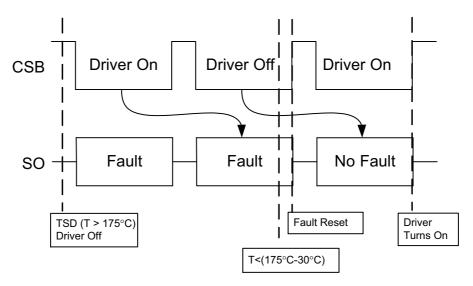
Figure 33. Thermal Shutdown Timing Diagram
