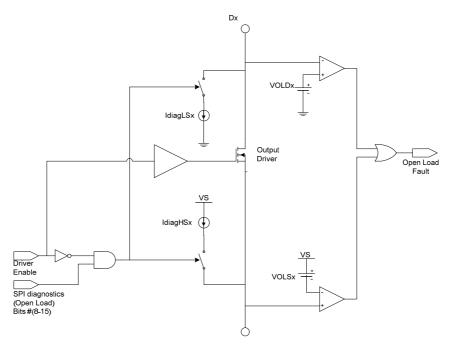
Figure 27. Open Load Diagnostic Principle
