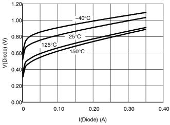
Figure 20. Source-to-Drain Voltage Body Diode
