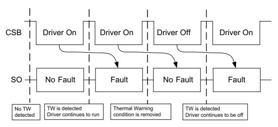
Figure 32. Thermal Warning Timing Diagram
