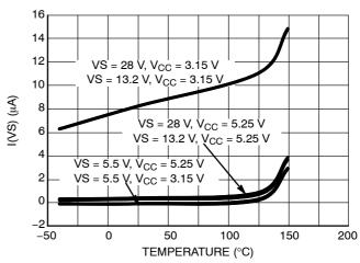
Figure 17. VS Standby Current vs. Temperature
