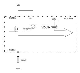
Figure 29. Open Load Circuitry as High Side Driver
