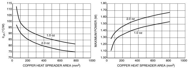
Figure 35.  $\theta_{JA}$  vs. Copper Heat Spreader
