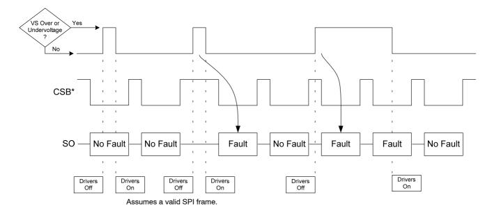
Figure 34. Power Supply Fail Timing Diagram
