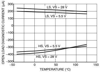
Figure 18. Open Load Detect Current vs.
