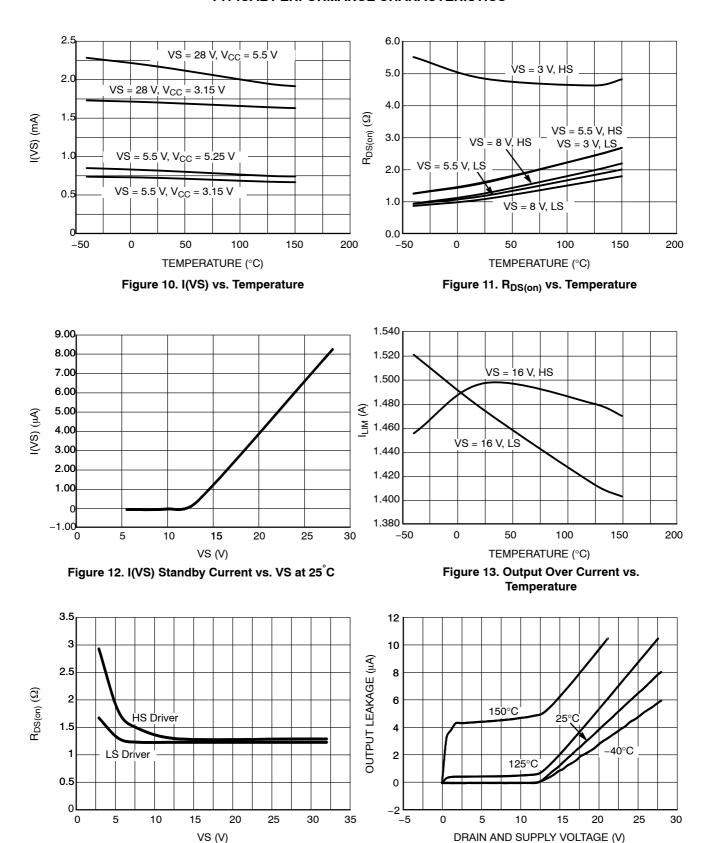
Figure 14. R<sub>DS(on)</sub> vs. VS
