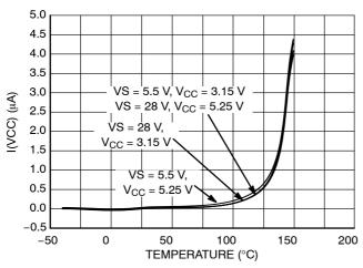
Figure 16. I(VCC) vs. Temperature
