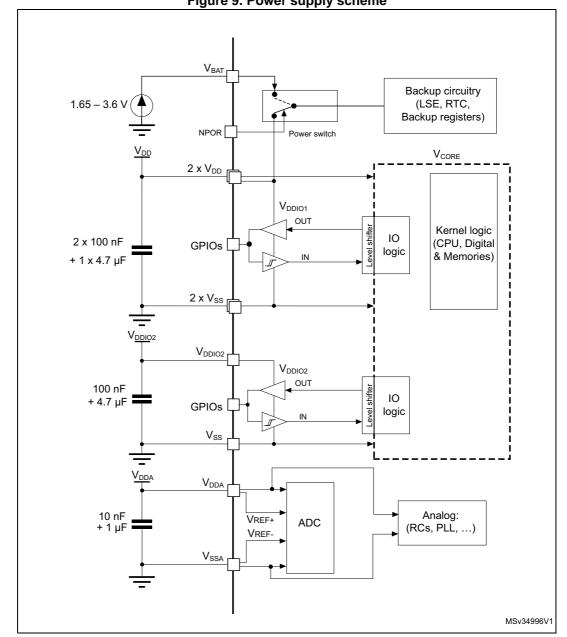
Figure 9. Power supply scheme
