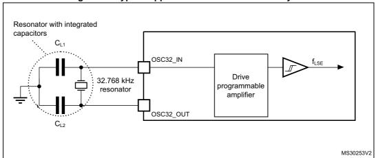
Figure 14. Typical application with a 32.768 kHz crystal
