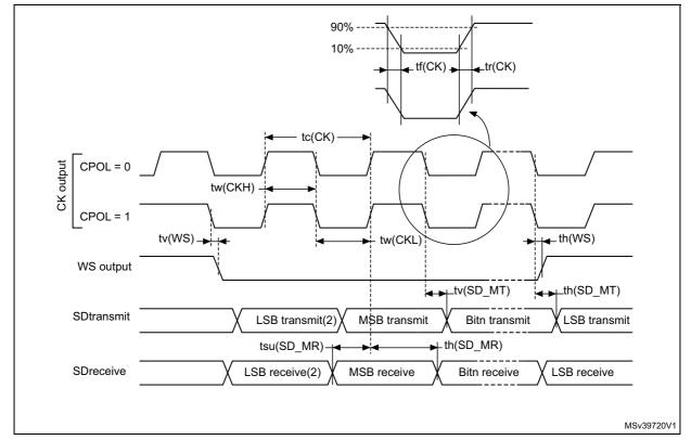
Figure 28. I<sup>2</sup>S master timing diagram (Philips protocol)
