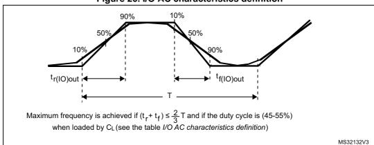
Figure 20. I/O AC characteristics definition
