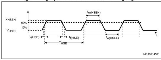
Figure 11. High-speed external clock source AC timing diagram
