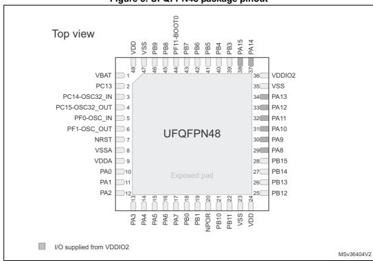
Figure 3. UFQFPN48 package pinout
