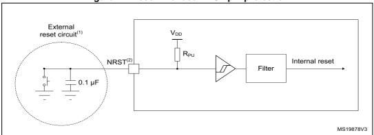
Figure 21. Recommended NRST pin protection
