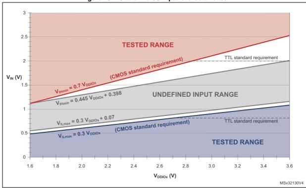
Figure 18. TC and TTa I/O input characteristics
