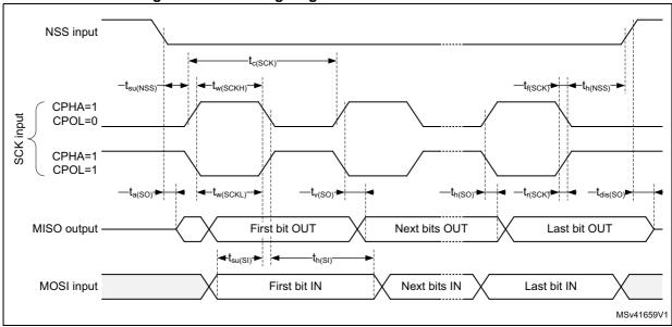
1. Measurement points are done at CMOS levels: 0.3  $V_{\rm DD}$  and 0.7  $V_{\rm DD}$ .
