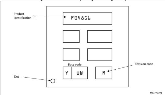
Figure 37. UFQFPN28 package marking example
