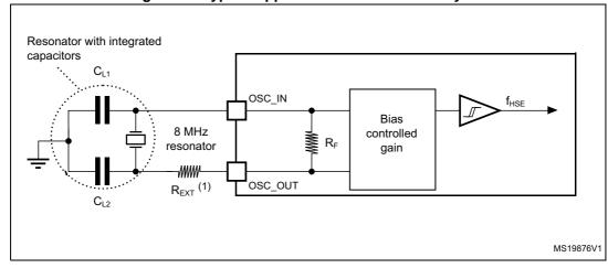
Figure 13. Typical application with an 8 MHz crystal
