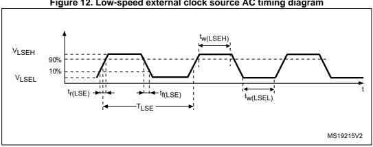
Figure 12. Low-speed external clock source AC timing diagram
