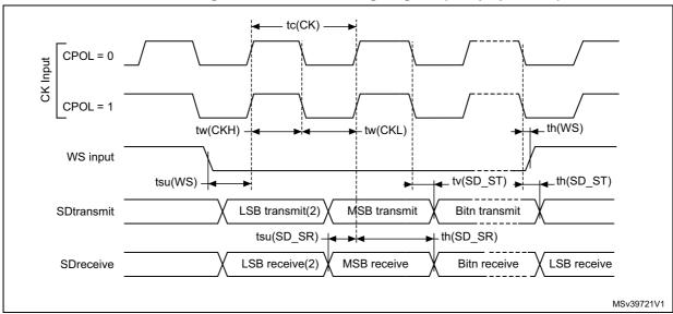
Figure 27. I<sup>2</sup>S slave timing diagram (Philips protocol)
