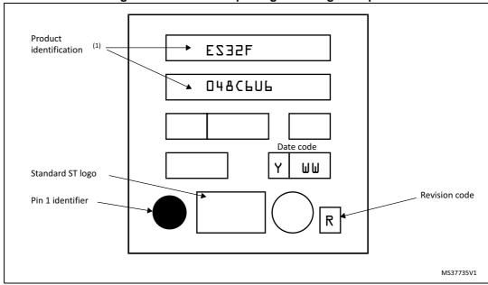
Figure 31. UFQFPN48 package marking example
