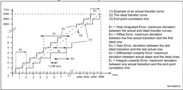
Figure 22. ADC accuracy characteristics
