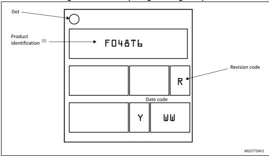
Figure 34. WLCSP36 package marking example
