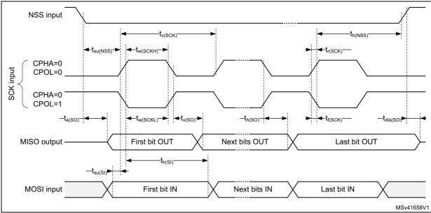
Figure 24. SPI timing diagram - slave mode and CPHA = 0
