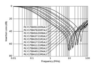
Common Mode Insertion Loss-Frequency Characteristics
