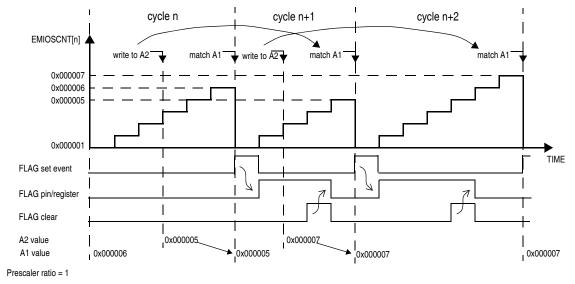
Figure 27-32. Modulus Counter Buffered (MCB) Up Count mode
