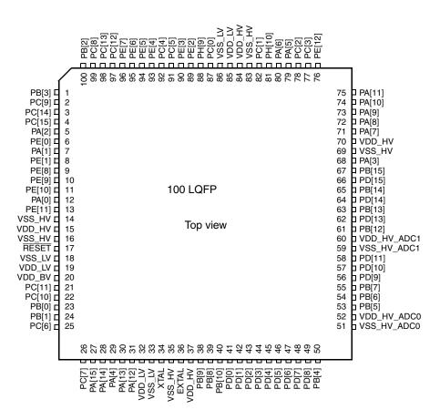
Figure 4-1. 100-pin LQFP pinout
