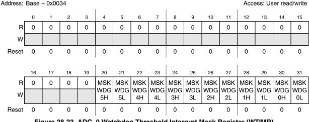
Figure 28-23. ADC\_0 Watchdog Threshold Interrupt Mask Register (WTIMR)
