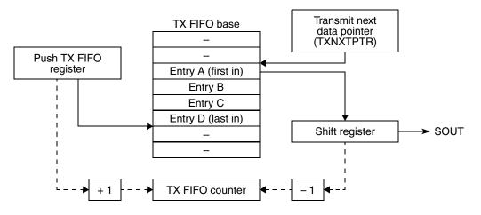
Figure 26-25. TX FIFO pointers and counter
