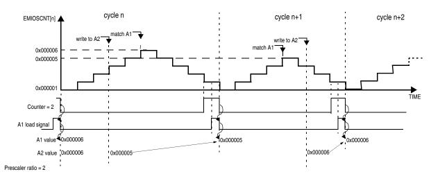
Figure 27-35. MCB Mode A1 Register Update in Up/Down Counter mode
