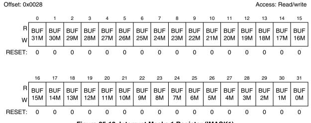
Figure 25-12. Interrupt Masks 1 Register (IMASK1)
