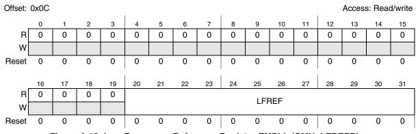
Figure 6-15. Low Frequency Reference Register FMPLL (CMU\_LFREFR)
