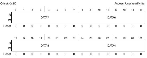
Figure 24-33. Buffer data register most significant (BDRM)
