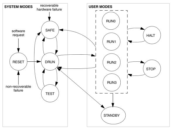
Figure 8-54. MC\_ME Mode Diagram
