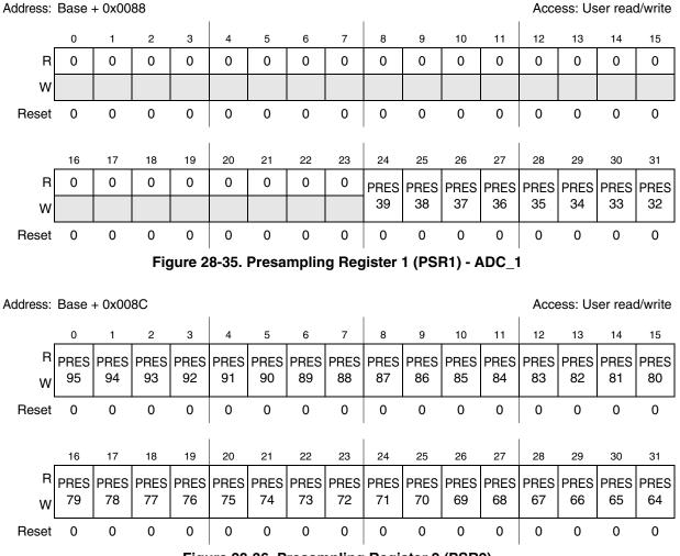
Figure 28-36. Presampling Register 2 (PSR2)
