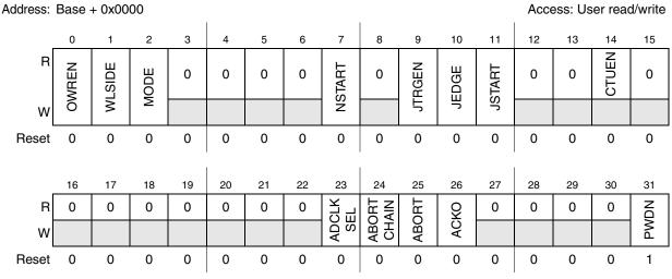
Figure 28-9. Main Configuration Register (MCR)
