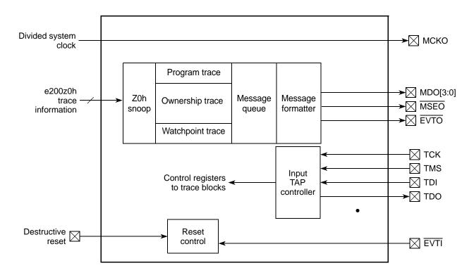
Figure 36-1. NDI functional block diagram
