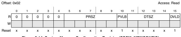
Figure 5-14. System Memory Configuration Register (SSCM\_MEMCONFIG)
