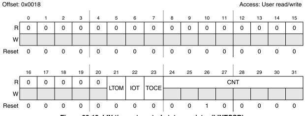
Figure 23-12. LIN timeout control status register (LINTCSR)
