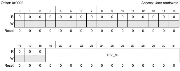
Figure 23-16. LIN integer baud rate register (LINIBRR)
