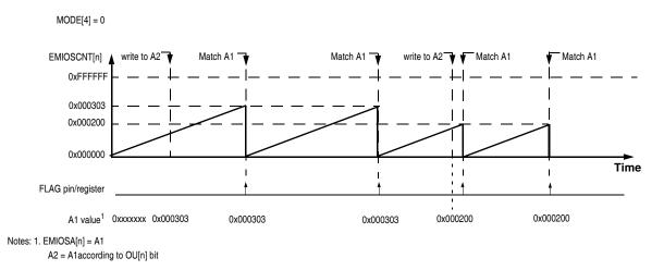
Figure 27-30. Modulus Counter Up mode example
