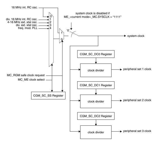
Figure 7-6. MC\_CGM System Clock Generation Overview
