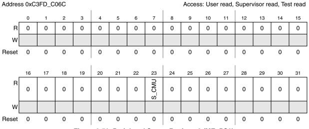
Figure 8-50. Peripheral Status Register 3 (ME\_PS3)
