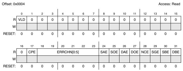
Figure 16-3. DMA Error Status (EDMA\_ESR) Register
