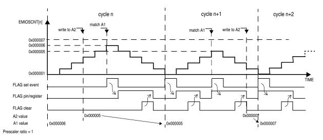
Figure 27-33. Modulus Counter Buffered (MCB) Up/Down mode
