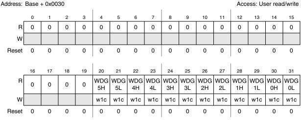
Figure 28-21. ADC\_0 Watchdog Threshold Interrupt Status Register (WTISR)
