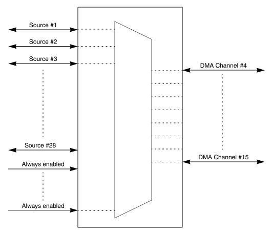
Figure 17-6. DMA\_MUX channel 4–15 block diagram
