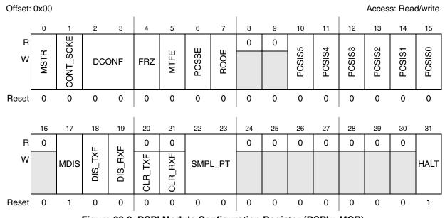
Figure 26-3. DSPI Module Configuration Register (DSPIx\_MCR)
