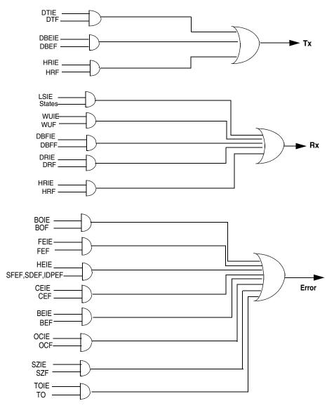
Figure 24-56. Interrupt diagram
