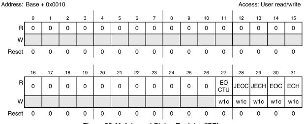
Figure 28-11. Interrupt Status Register (ISR)
