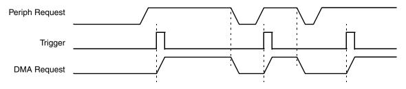
Figure 17-4. DMA\_MUX channel triggering: Normal operation
