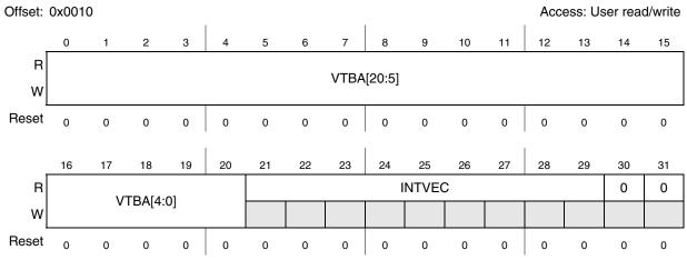
Figure 18-4. INTC Interrupt Acknowledge Register (INTC\_IACKR) when INTC\_MCR[VTES] = 0
