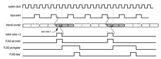
Note 1: When a match occurs, the first system clock cycle is used to clear the internal counter, and at the next edge of prescaler clock enable the counter will start counting.
