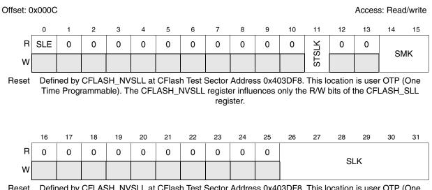
Reset Defined by CFLASH\_NVSLL at CFlash Test Sector Address 0x403DF8. This location is user OTP (One Time Programmable). The CFLASH\_NVSLL register influences only the R/W bits of the CFLASH\_SLL register.
