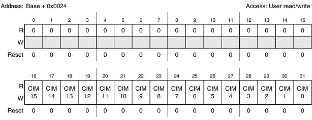
Figure 28-17. Channel Interrupt Mask Register 0 (CIMR0)
