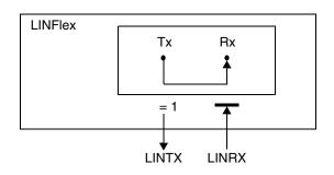
Figure 23-5. LINFlex in self test mode
