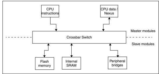
Figure 19-1 shows a block diagram of the crossbar switch.
