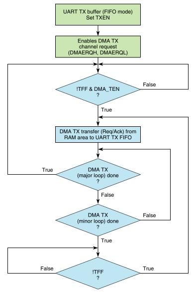
Figure 24-52. FSM to control the DMA TX interface (UART node)
