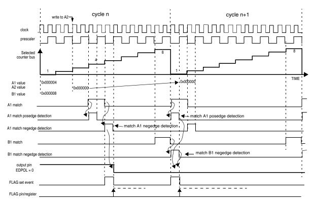
Figure 27-45. OPWMB mode with 0% duty cycle
