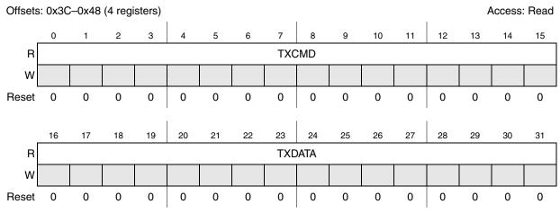
Figure 26-10. DSPI Transmit FIFO Register 0–3 (DSPIx\_TXFRn)
