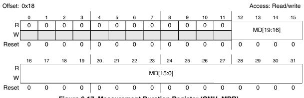
Figure 6-17. Measurement Duration Register (CMU\_MDR)
