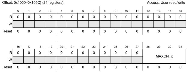
Figure 21-13. Interrupt Filter Maximum Counter Registers (IFMC0–IFMC23)
