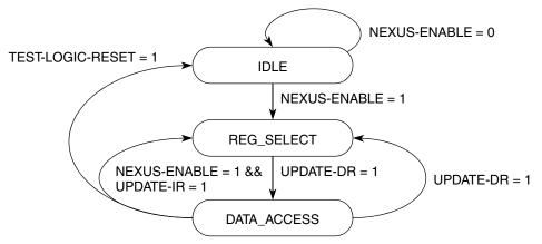
Figure 36-8. NEXUS Controller State Machine
