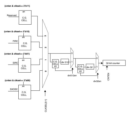
Figure 13-2. Clock gating for RTC clocks
