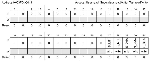
Figure 8-37. Invalid Mode Transition Status Register (ME\_IMTS)
