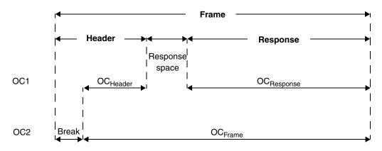
Figure 23-32. Header and response timeout
