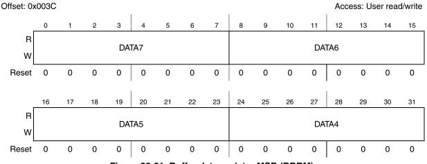
Figure 23-21. Buffer data register MSB (BDRM)
