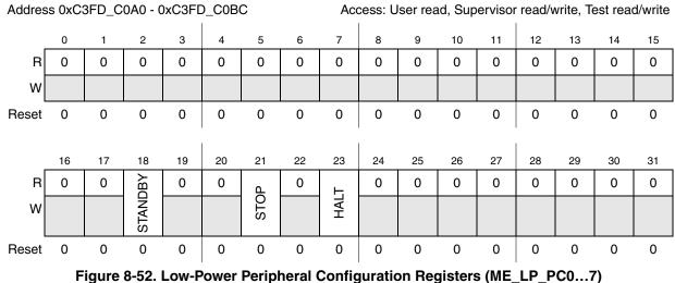
Figure 6-52. Low-Power Peripheral Configuration Registers (MC\_LP\_PC0...7)
