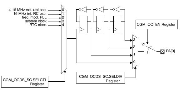
Figure 7-7. MC\_CGM Output Clock Multiplexer and PA[0] Generation
