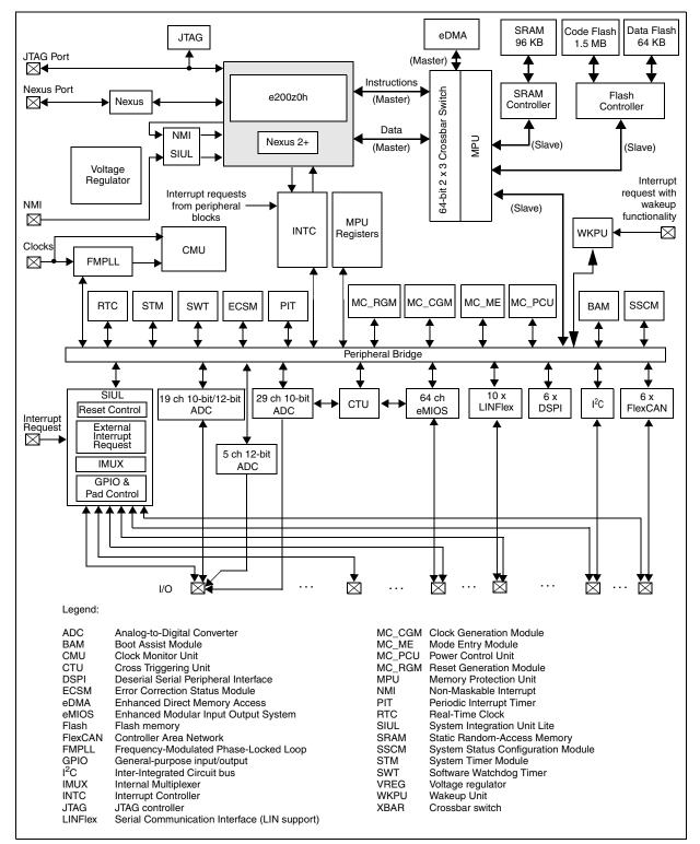
Figure 2. MPC5607B block diagram
