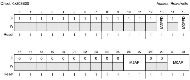
Figure 30-45. Nonvolatile Platform Flash Access Protection Register (NVPFAPR)
