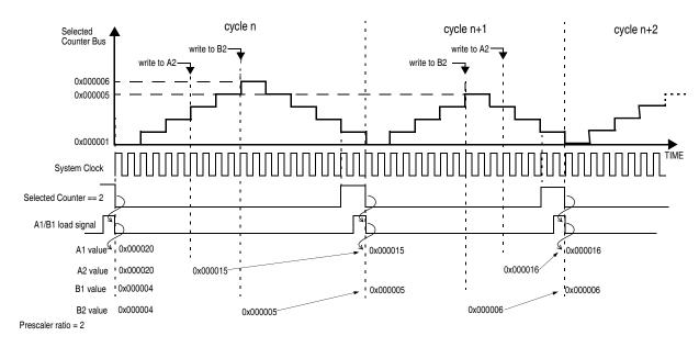
Figure 27-40. OPWMCB A1 and B1 registers load
