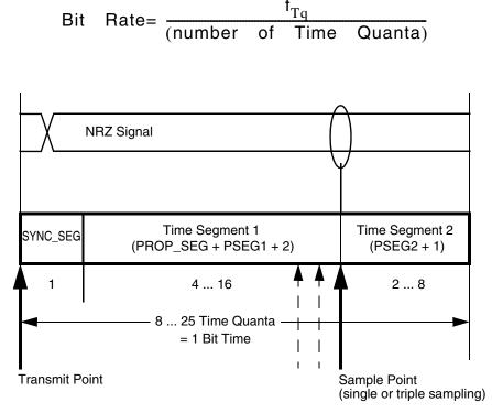
Figure 25-17. Segments within the Bit Time
