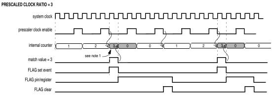
Note 1: When a match occurs, the first clock cycle is used to clear the internal counter, and only after a second edge of pre scaled clock the counter will start counting.
