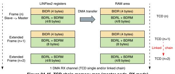
Figure 24-45. TCD chain memory map (master node, RX mode)
