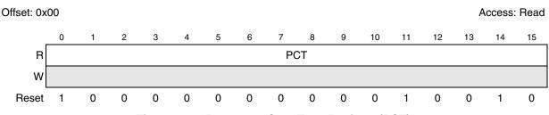
Figure 34-1. Processor Core Type Register (PCT)
