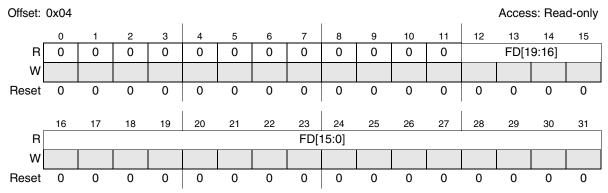
Figure 6-13. Frequency Display Register (CMU\_FDR)
