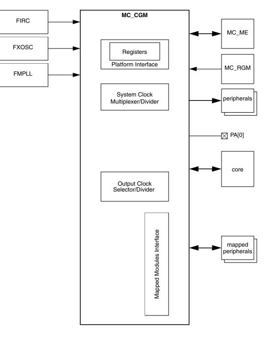
Figure 7-1. MC\_CGM block diagram
