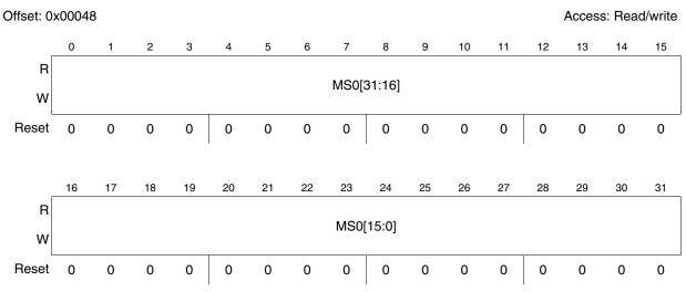
Figure 30-16. CFlash User Multiple Input Signature Register 0 (CFLASH\_UMISR0)
