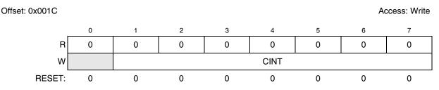
Figure 16-10. DMA Clear Interrupt Request (EDMA\_CIRQR) Fields
