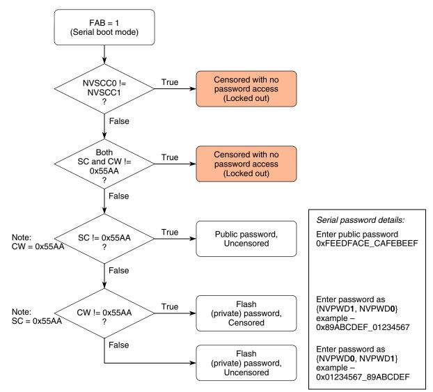
Figure 5-5. Censorship control in serial boot mode
