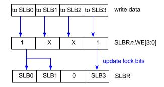
Figure 32-8. Change Lock Settings for Mixed Protection
