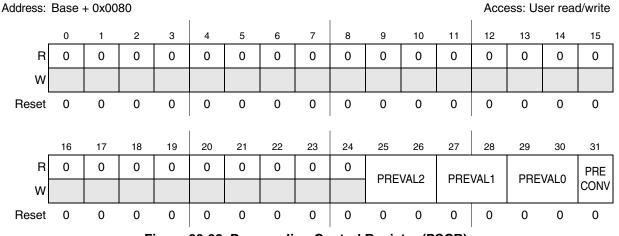
Figure 28-32. Presampling Control Register (PSCR)
