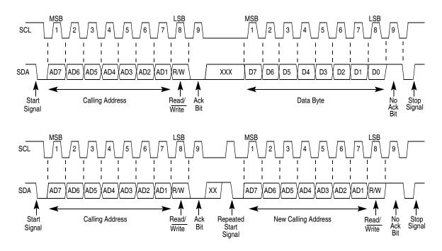
Figure 22-11. I<sup>2</sup>C bus transmission signals
