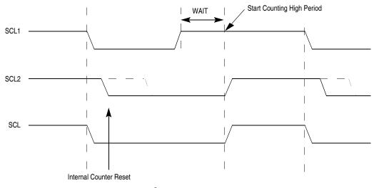
Figure 22-13. I<sup>2</sup>C bus clock synchronization
