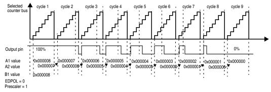
Figure 27-46. OPWMB mode from 100% to 0% duty cycle
