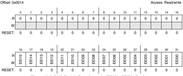
Figure 16-5. DMA Enable Error Interrupt (EDMA\_EEIRL) Register
