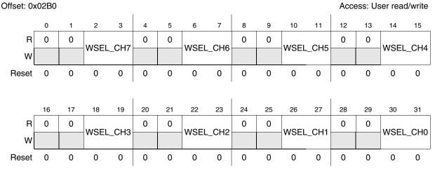
Figure 28-60. Channel Watchdog Select Register 0 (CWSELR0) – ADC\_1
