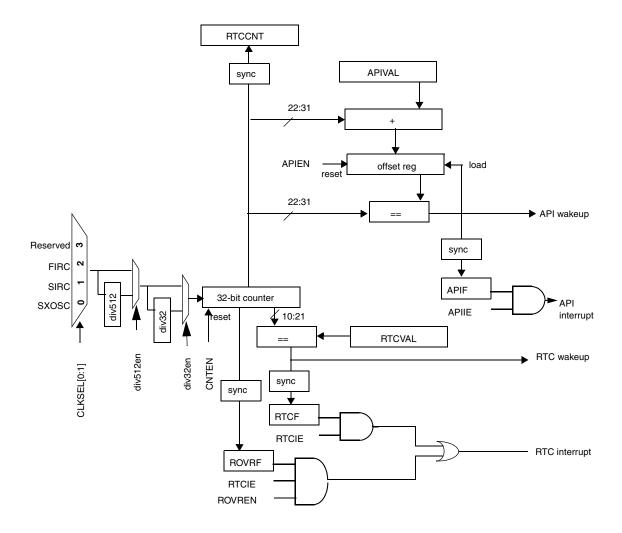
Figure 13-1. RTC/API block diagram
