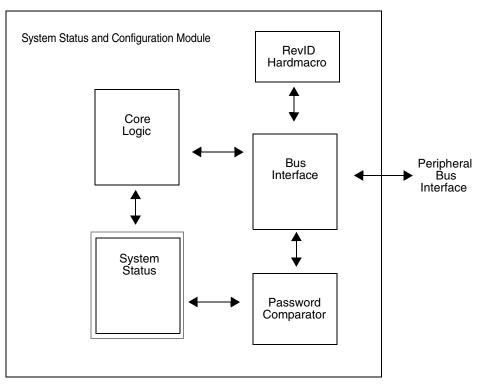
Figure 5-12. SSCM block diagram
