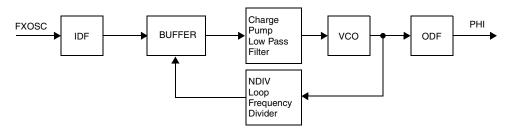
Figure 6-6. FMPLL block diagram
