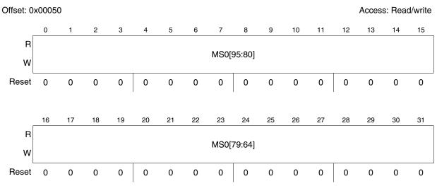
Figure 30-18. CFlash User Multiple Input Signature Register 2 (CFLASH\_UMISR2)
