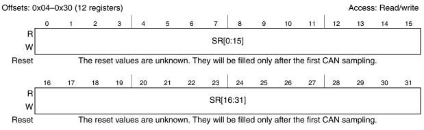
Figure 14-3. CAN Sampler Sample Registers 0–11
