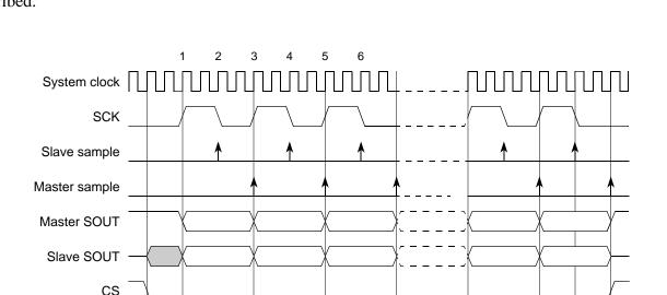
Figure 26-19 shows the modified transfer format for CPHA = 1. Only the condition where CPOL = 0 is described.
