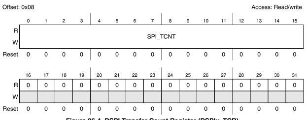
Figure 26-4. DSPI Transfer Count Register (DSPIx\_TCR)
