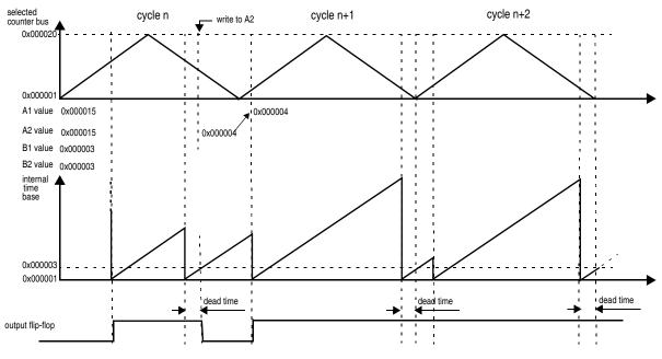
Figure 27-43. OPWMCB with 100% Duty Cycle (A1 = 4 and B1 = 3)
