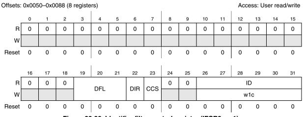
Figure 23-26. Identifier filter control register (IFCR2n + 1)
