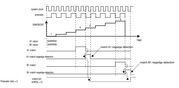
Figure 27-36. OPWFMB A1 and B1 match to Output Register Delay
