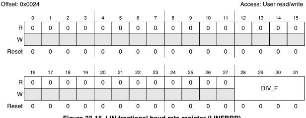
Figure 23-15. LIN fractional baud rate register (LINFBRR)
