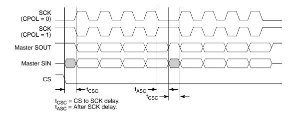
Figure 26-21. Example of continuous transfer (CPHA = 1, CONT = 1)
