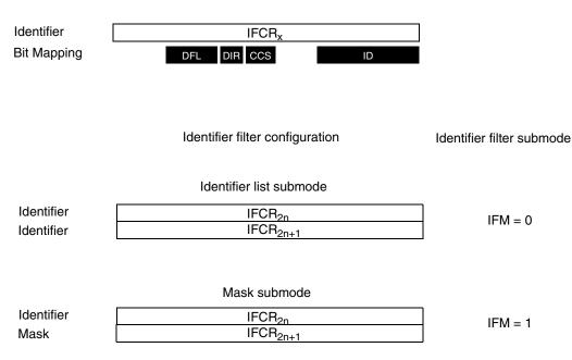
Figure 24-9. Filter configuration - register organization
