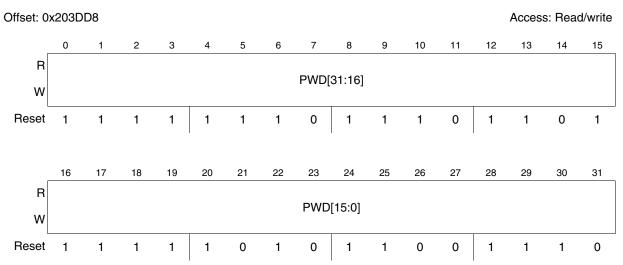
Figure 30-21. CFlash Nonvolatile Private Censorship Password 0 Register (NVPWD0)
