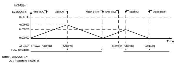
Figure 27-31. Modulus Counter Up/Down mode example
