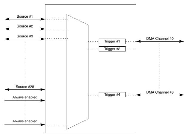
Figure 17-3. DMA\_MUX channel 0–3 block diagram
