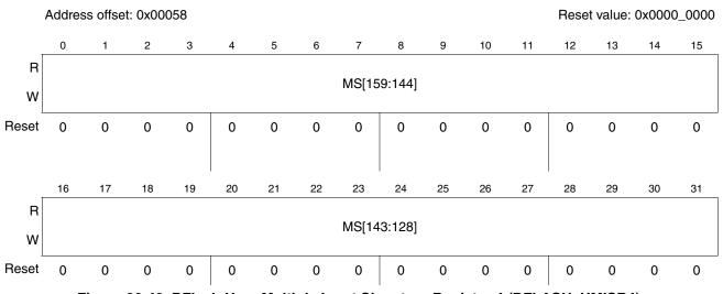
Figure 30-40. DFlash User Multiple Input Signature Register 4 (DFLASH\_UMISR4)
