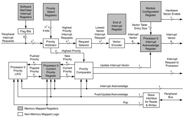
Figure 18-1. INTC block diagram
