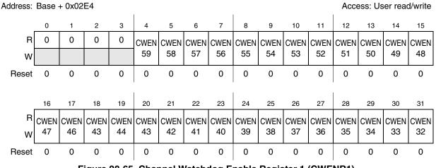
Figure 28-65. Channel Watchdog Enable Register 1 (CWENR1)
