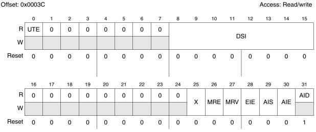
Figure 30-33. DFlash User Test 0 register (DFLASH\_UT0)
