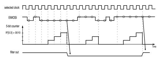
Figure 27-51. Input programmable filter example
