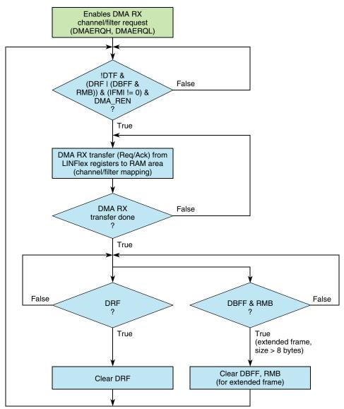
Figure 24-50. FSM to control the DMA RX interface (slave node)
