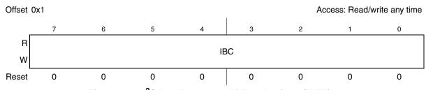
Figure 22-3. I<sup>2</sup>C Bus Frequency Divider Register (IBFD)
