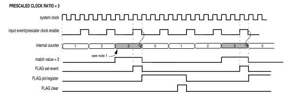
Note 1: The match occurs only when the input event/prescaler clock enable is active. Then, the internal counter is immediately cleared.
