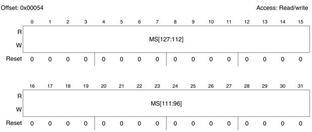
Figure 30-19. CFlash User Multiple Input Signature Register 3 (CFLASH\_UMISR3)
