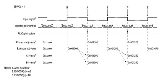
Figure 27-23. Input pulse width measurement example
