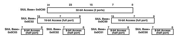
Figure 21-15. Data Port example arrangement showing configuration for different port width accesses
