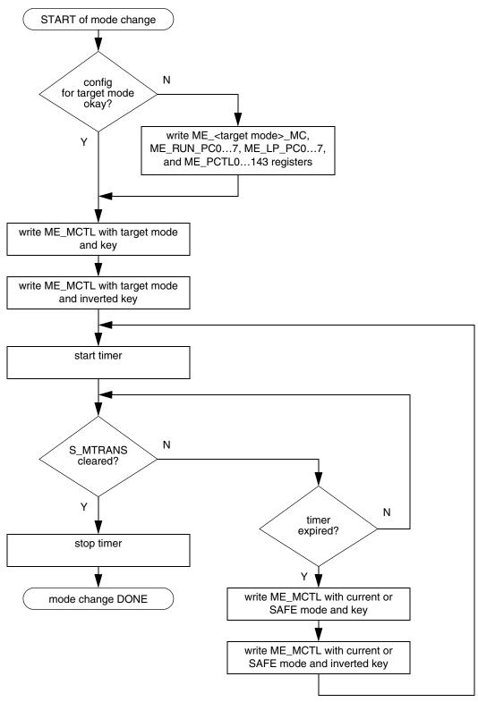
Figure 8-56. MC\_ME Application Example Flow Diagram
