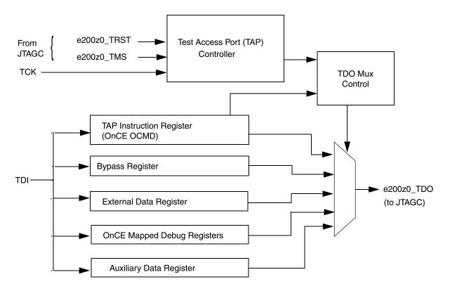
Figure 35-6. e200z0 OnCE Block Diagram
