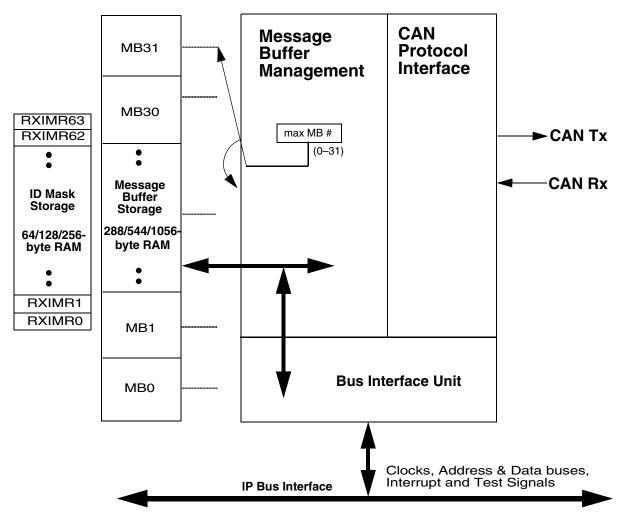
Figure 25-1. FlexCAN block diagram
