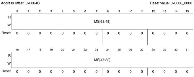
Figure 30-37. DFlash User Multiple Input Signature Register 1 (DFLASH\_UMISR1)
