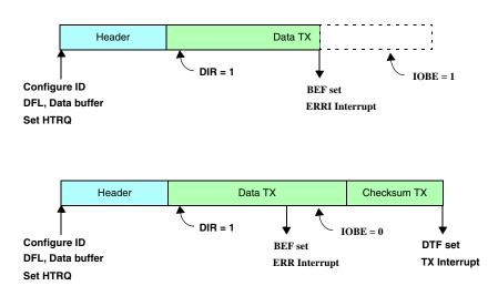
Figure 24-59. Programming consideration: master node, transmitter, bit error
