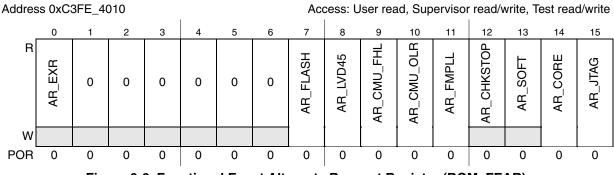
Figure 9-6. Functional Event Alternate Request Register (RGM\_FEAR)
