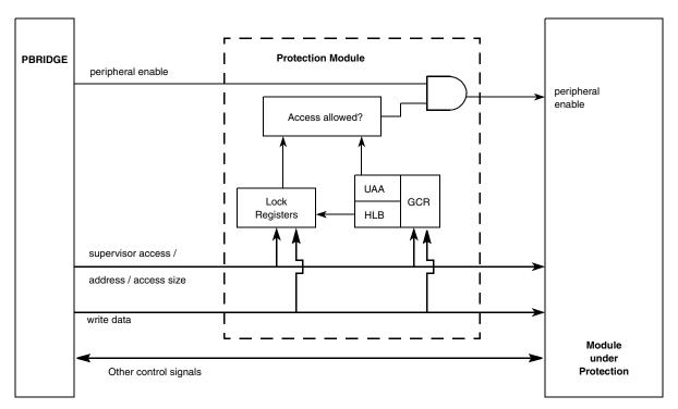
Figure 32-1. Register Protection block diagram
