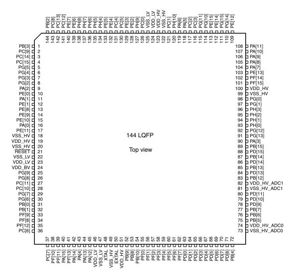
Figure 4-2. 144-pin LQFP pinout
