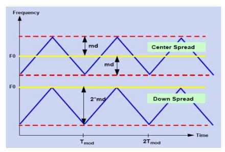
Figure 6-10. Frequency modulation
