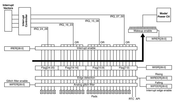
Figure 12-12. External interrupt pad diagram
