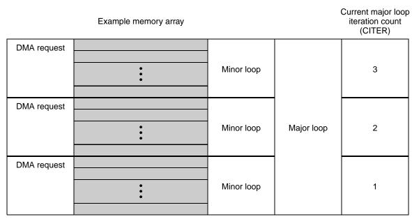
Figure 16-22. Example of multiple loop iterations
