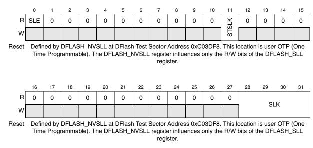
Figure 30-29. DFlash Secondary Low/mid address space block Locking register (DFLASH\_SLL)
