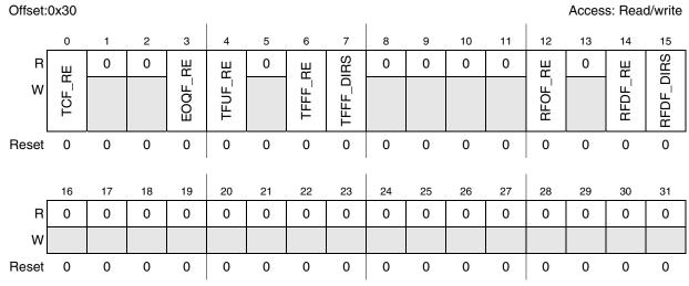
Figure 26-7. DSPI DMA / Interrupt Request Select and Enable Register (DSPIx\_RSER)
