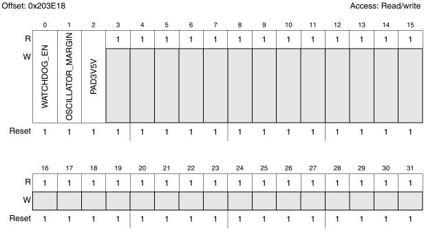
Figure 30-25. CFlash Nonvolatile User Options register (NVUSRO)
