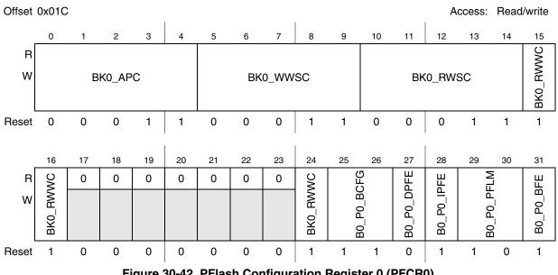
Figure 30-42. PFlash Configuration Register 0 (PFCR0)
