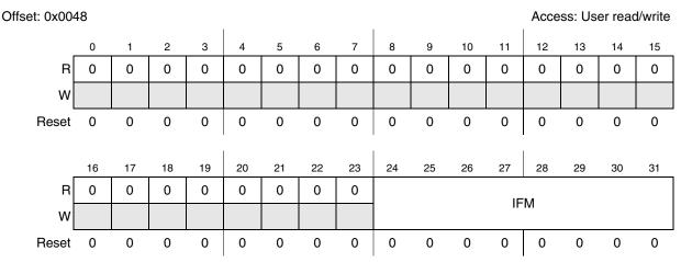
Figure 23-24. Identifier filter mode register (IFMR)
