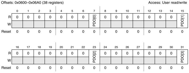
Figure 21-11. Port GPIO Pad Data Output Register 0-3 (GPDO0\_3)
