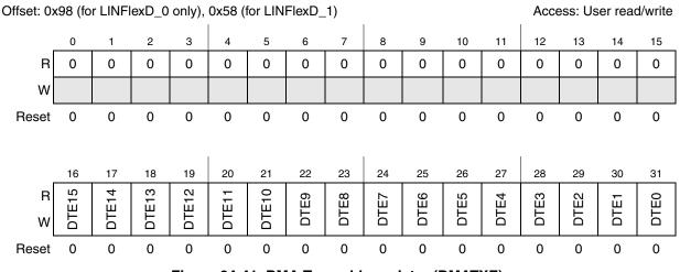
Figure 24-41. DMA Tx enable register (DMATXE)
