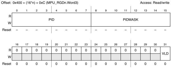
Figure 20-8. MPU Region Descriptor, Word 3 Register (MPU\_RGDn.Word3)
