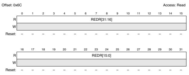
Figure 34-18. Platform RAM ECC Data Register (PREDR)
