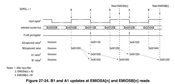
Reading EMIOSA[n] followed by EMIOSB[n] always provides coherent data. If not coherent data is required for any reason, the sequence of reads should be inverted, therefore EMIOSB[n] should be read prior to EMIOSA[n] register. Note that even in this case B1 register updates will be blocked after EMIOSA[n] read, thus a second EMIOSB[n] is required in order to release B1 register updates.
