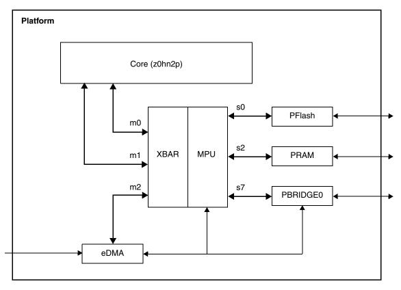
Figure 20-1. MPU block diagram
