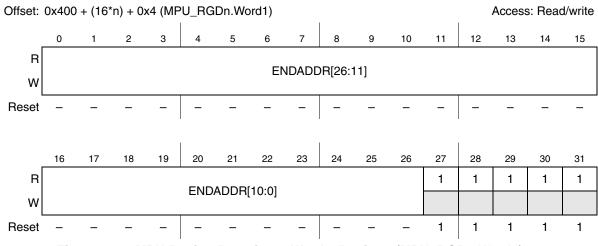
Figure 20-6. MPU Region Descriptor, Word 1 Register (MPU\_RGDn.Word1)
