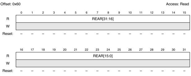
Figure 34-14. Platform RAM ECC Address Register (PREAR)
