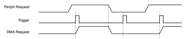
Figure 17-5. DMA\_MUX channel triggering: Ignored trigger
