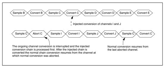
Figure 28-3. Injected sample/conversion sequence
