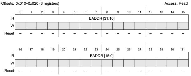
Figure 20-3. MPU Error Address Register, Slave Port n (MPU\_EARn)
