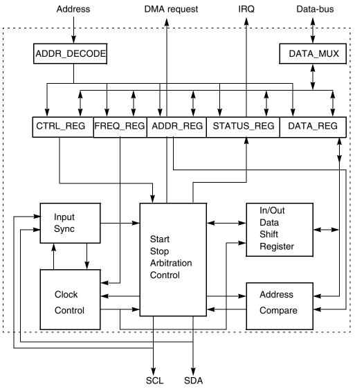
Figure 22-10. I<sup>2</sup>C module DMA interface block diagram
