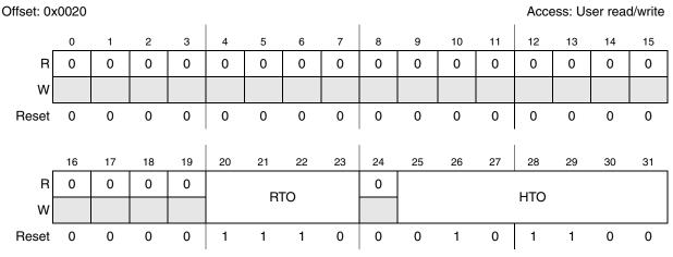
Figure 23-14. LIN timeout control register (LINTOCR)
