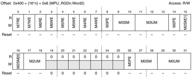
Figure 20-7. MPU Region Descriptor, Word 2 Register (MPU\_RGDn.Word2)
