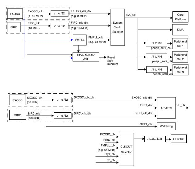
Figure 6-1. MPC5607B system clock generation
