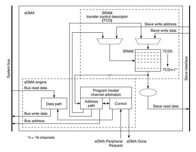
Figure 16-1. eDMA block diagram
