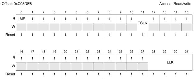
Figure 30-28. DFlash Nonvolatile Low/Mid address space block Locking register (DFLASH\_NVLML)
