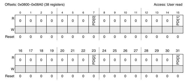
Figure 21-12. Port GPIO Pad Data Input Register 0-3 (GPDI0\_3)
