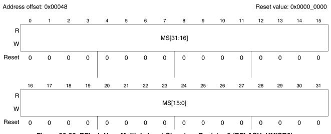
Figure 30-36. DFlash User Multiple Input Signature Register 0 (DFLASH\_UMISR0)
