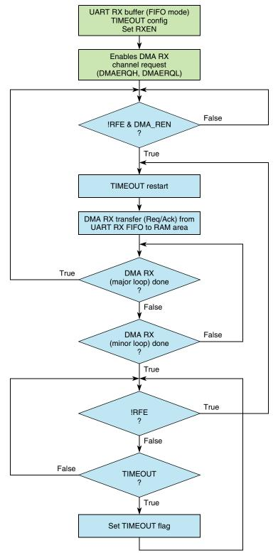
Figure 24-54. FSM to control the DMA RX interface (UART node)
