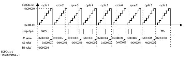
Figure 27-39. OPWFMB mode from 100% to 0% duty cycle
