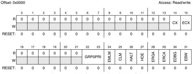
Figure 16-2. DMA Control Register (EDMA\_CR)
