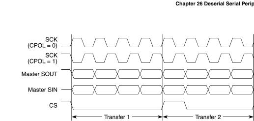
Figure 26-24. Continuous SCK timing diagram (CONT=1)
