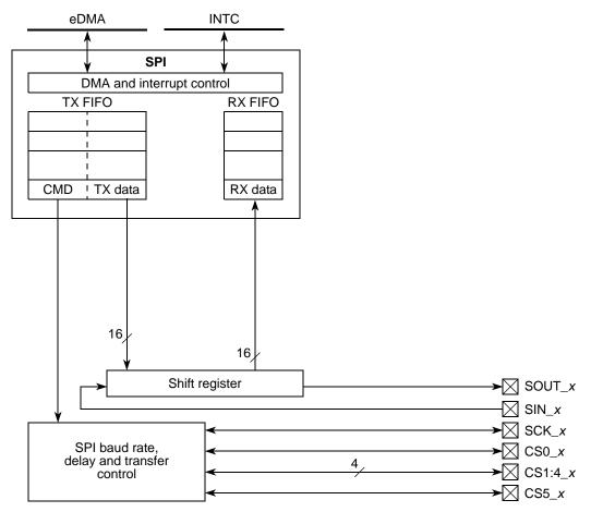
Figure 26-1. DSPI block diagram
