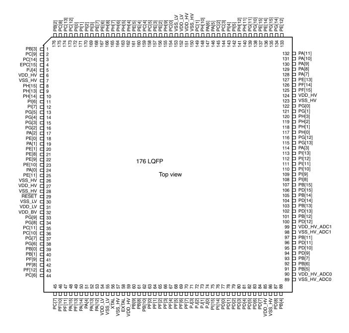
Figure 4-3. 176-pin LQFP pinout
