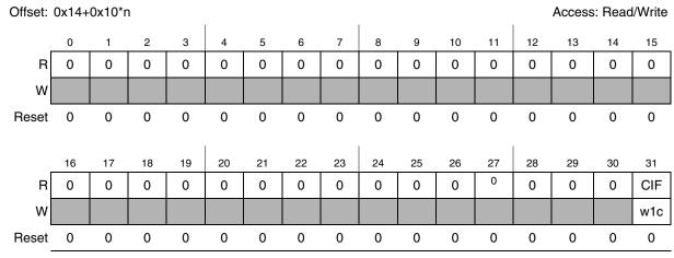
Figure 27-5. STM Channel Interrupt Register (STM\_CIRn)
