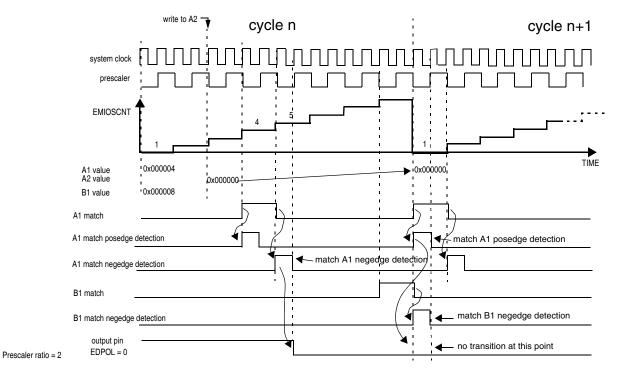
Figure 27-37. OPWFMB Mode with A1 = 0 (0% duty cycle)
