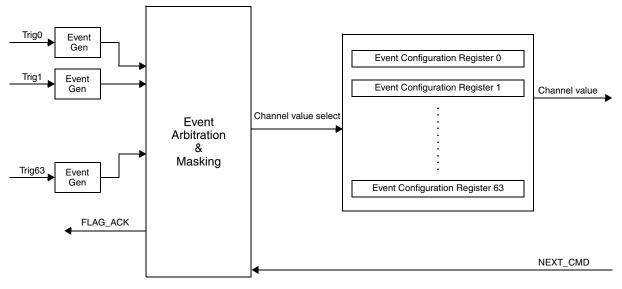
Figure 29-1. Cross Triggering Unit block diagram
