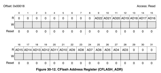
The CFLASH\_ADR provides the first failing address in the event module failures (ECC or FPEC) occur or the first address at which an ECC single error correction occurs.
