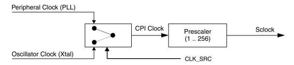
Figure 25-16. CAN Engine Clocking Scheme
