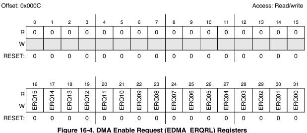
ure 16-4. DMA Enable Request (EDMA\_ERQRL) Registe
