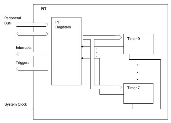
Figure 27-56. PIT block diagram
