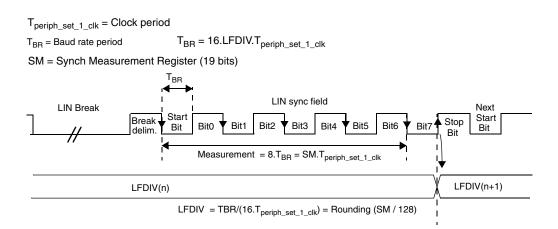
Figure 24-11. LIN sync field measurement
