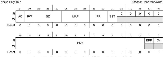
Figure 36-14. Read/Write Access Control/Status Register (RWCS)
