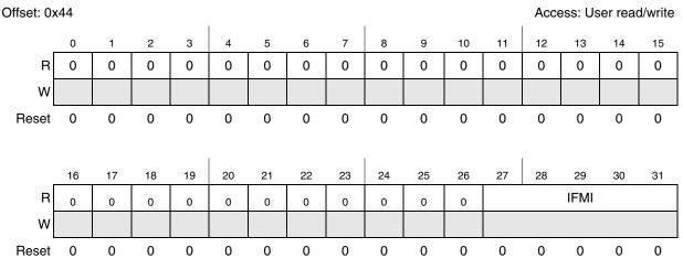
Figure 24-35. Identifier filter match index (IFMI)
