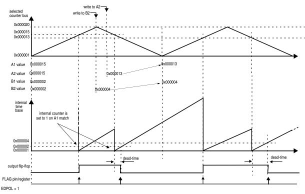
Figure 27-42. OPWMCB with trail dead time insertion
