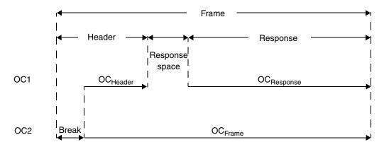
Figure 24-55. Header and response timeout
