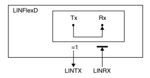
Figure 24-13. LINFlexD in Self Test mode
