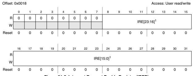
Figure 21-5. Interrupt Request Enable Register (IRER)
