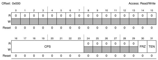
Figure 27-2. STM Control Register (STM\_CR)
