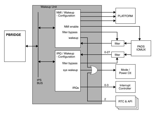
Figure 12-1. WKPU block diagram
