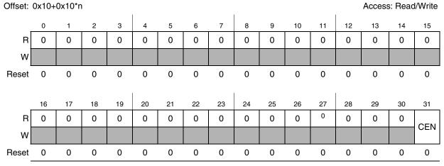
Figure 27-4. STM Channel Control Register (STM\_CCRn)
