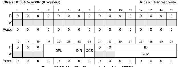
Figure 23-25. Identifier filter control register (IFCR2n)
