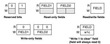
Figure 1-1. Register figure conventions
