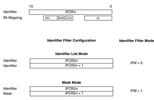
Figure 23-29. Filter configuration—register organization
