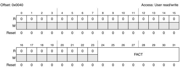
Figure 23-22. Identifier filter enable register (IFER)
