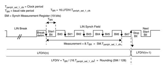
Figure 23-31. LIN synch field measurement
