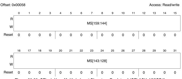
Figure 30-20. CFlash User Multiple Input Signature Register 4 (CFLASH\_UMISR4)
