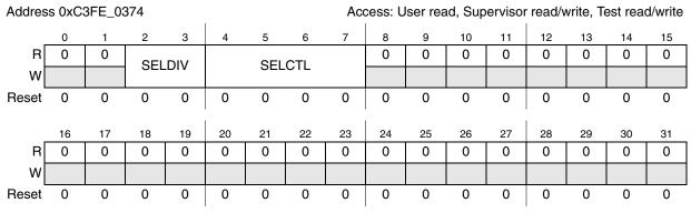
Figure 7-3. Output Clock Division Select Register (CGM\_OCDS\_SC)
