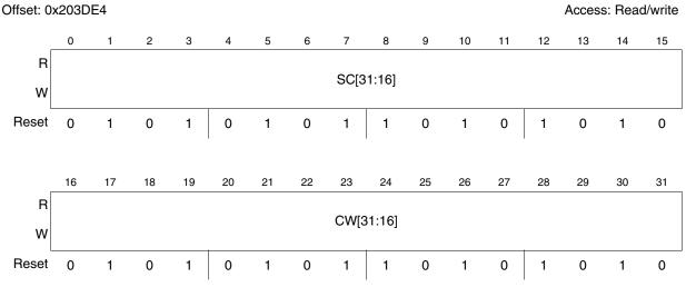
Figure 30-24. CFlash Nonvolatile System Censorship Control 1 register (NVSCC1)
