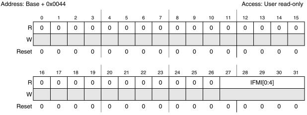
Figure 23-23. Identifier filter match index (IFMI)
