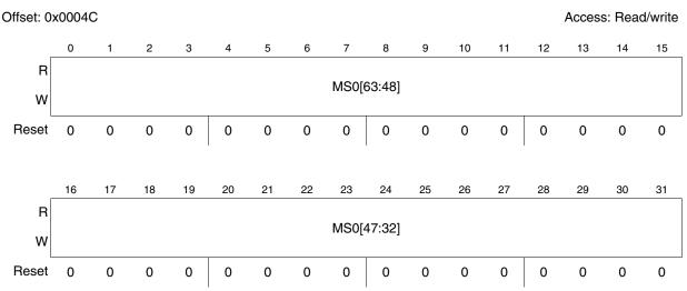
Figure 30-17. CFlash User Multiple Input Signature Register 1 (CFLASH\_UMISR1)
