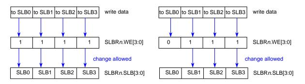
Figure 32-5. Change Lock Settings Directly Via Area #4
