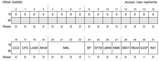
Figure 23-6. LIN control register 1 (LINCR1)
