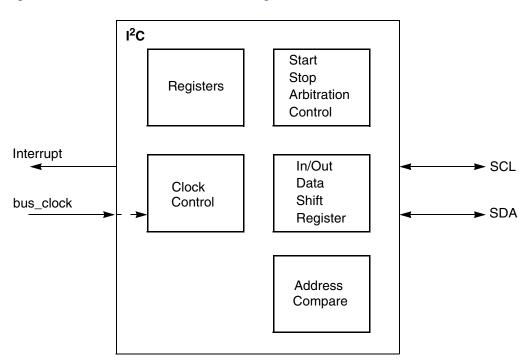
Figure 22-1. I<sup>2</sup>C block diagram
