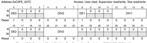
Figure 7-5. System Clock Divider Configuration Registers (CGM\_SC\_DC0...2)
