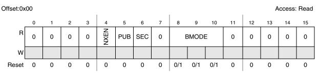
Figure 5-13. System Status Register (SSCM\_STATUS)
