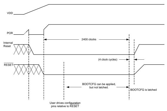
Figure 9-12. Reset configuration timing
