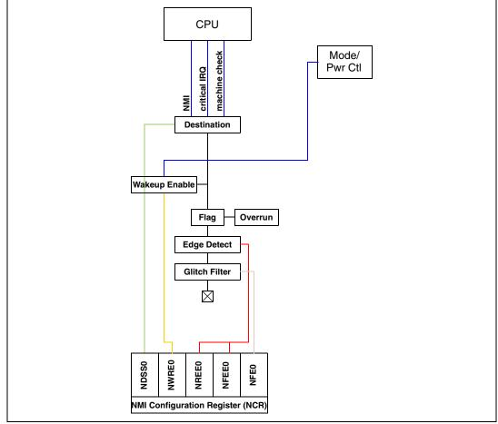
Figure 12-11. NMI pad diagram
