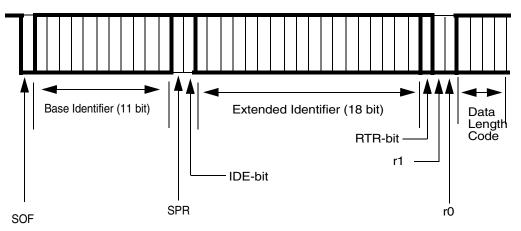
Figure 14-1. Extended CAN data frame
