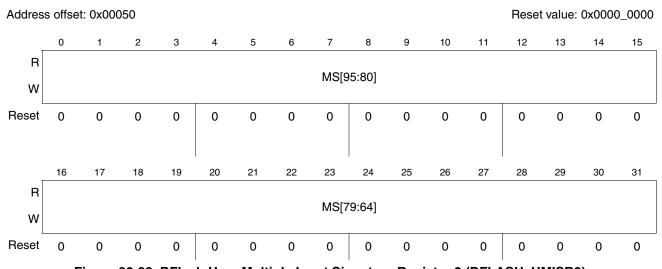
Figure 30-38. DFlash User Multiple Input Signature Register 2 (DFLASH\_UMISR2)
