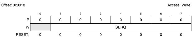
Figure 16-6. DMA Set Enable Request (EDMA\_SERQR) Register
