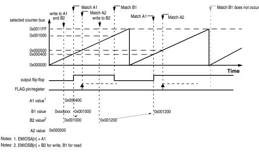
Figure 27-49. OPWMT with 100% duty cycle
