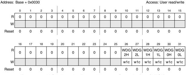
Figure 28-22. ADC\_1 Watchdog Threshold Interrupt Status Register (WTISR)
