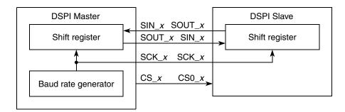
Figure 26-12. SPI serial protocol overview
