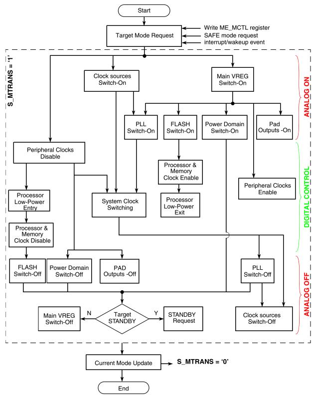
Figure 8-55. MC\_ME Transition Diagram
