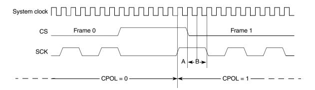
Figure 26-22. Polarity switching between frames
