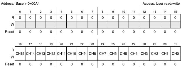
Figure 28-38. Normal Conversion Mask Register 0 (NCMR0)
