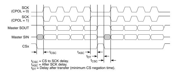
Figure 26-20. Example of non-continuous format (CPHA = 1, CONT = 0)
