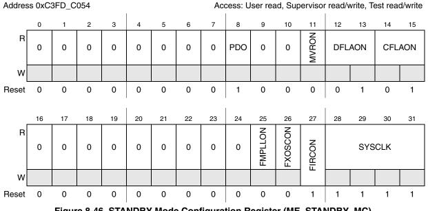
Figure 8-46. STANDBY Mode Configuration Register (ME\_STANDBY\_MC)
