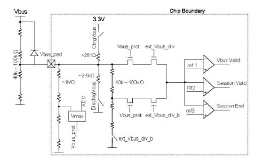
Figure 1. External Divider Schematic
