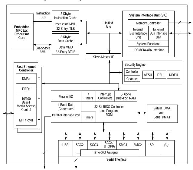
Figure 1. MPC885 Block Diagram
