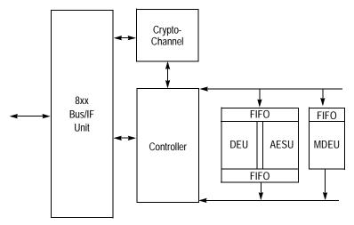
Figure 3. Security Engine Functional Blocks
