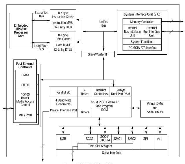
Figure 2. MPC880 Block Diagram
