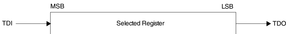
Figure 53-3. Shifting data through a register
