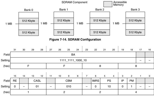
Figure 7-15. DACR Register Configuration
