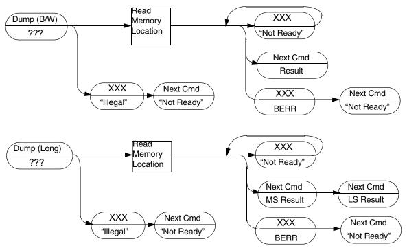
Figure 20-16. DUMP Memory Block Command Sequence
