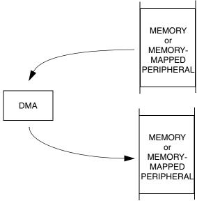
Figure 14-2. Dual Address Transfer
