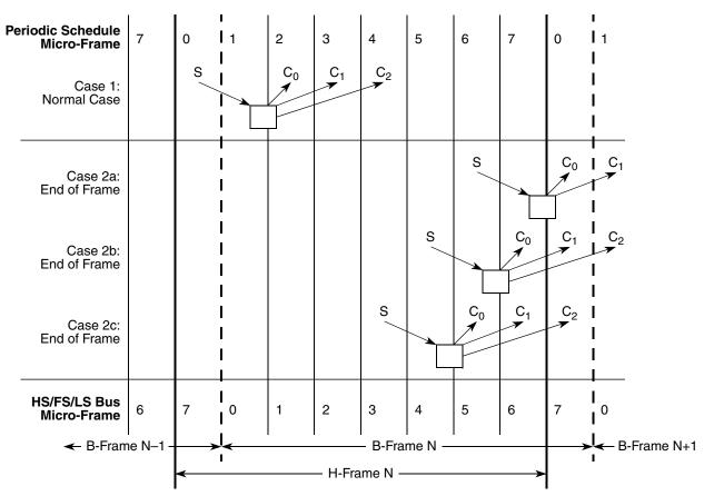
Figure 24-53. Split Transaction, Interrupt Scheduling Boundary Conditions
