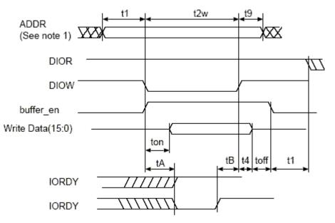
Figure 23-3. PIO Write Mode Timing
