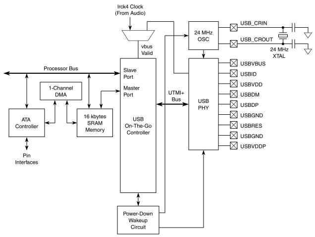
Figure 24-1. USB Interface Block Diagram
