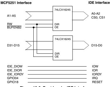
Figure 19-2. Boot Loader IDE Interface
