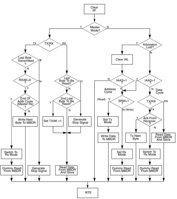
Figure 18-9. Flow-Chart of Typical I<sup>2</sup>C Interrupt Routine
