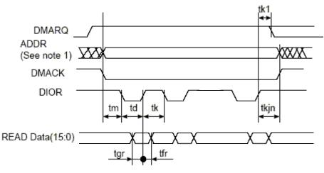
Figure 23-4. MDMA Read Timing
