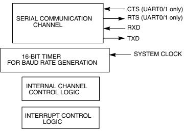
Figure 15-1. UART Block Diagram
