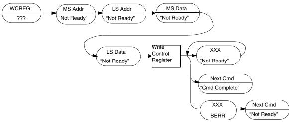
Figure 20-22. Write Control Register Command Sequence
