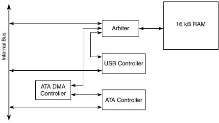
Figure 22-5. ATA/USB Shared RAM Block Diagram
