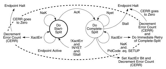
Figure 24-52. Host Controller Asynchronous Schedule Split-Transaction State Machine
