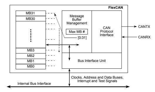
Figure 25-1. FlexCAN Block Diagram and Pinout
