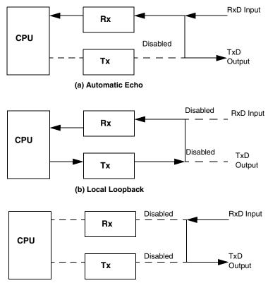
(c) Remote Loopback Figure 15-7. Looping Modes Functional Diagram
