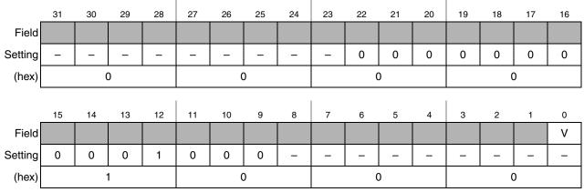
Figure 7-17. Mode Register Mapping to MCF5251 A[31:0]
