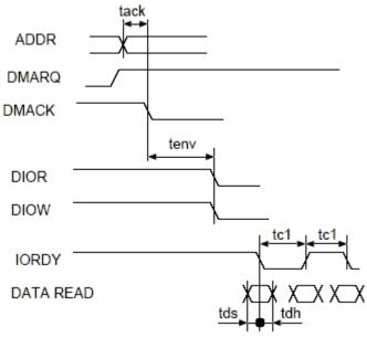
Figure 23-6. UDMA in Transfer Start Timing Diagram
