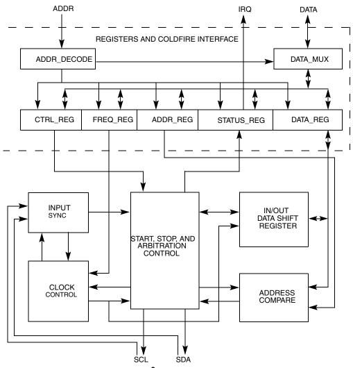
Figure 18-1. I<sup>2</sup>C Module Block Diagram
