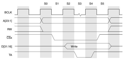
Figure 8-6 shows the description for the six states of a basic write cycle.
