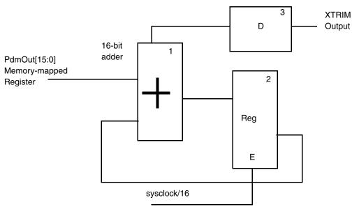
Figure 17-27. PDM Modulator Used on XTRIM Output
