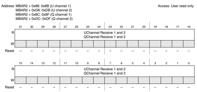
Figure 17-10. U Channel Receive and Q Channel Receive Registers
