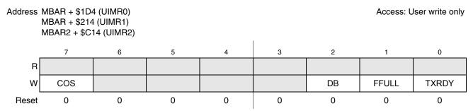
Figure 15-18. Interrupt Mask Register (UIMRn)
