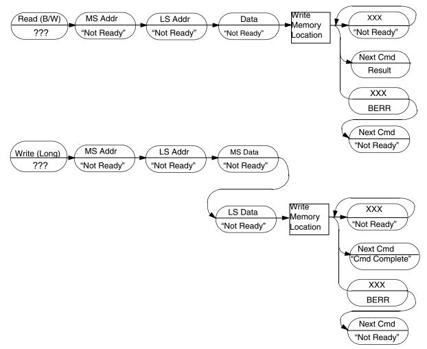
Figure 20-14. Write Memory Location Command Sequence
