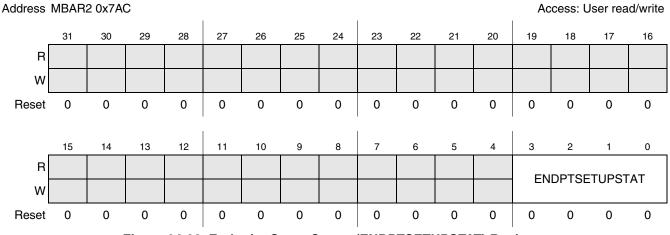
Figure 24-28. Endpoint Setup Status (ENDPTSETUPSTAT) Register
