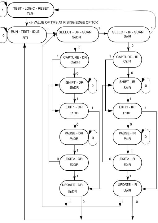
Figure 21-2. JTAG TAP Controller State Machine
