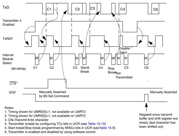
Figure 15-5. Transmitter Timing Diagram
