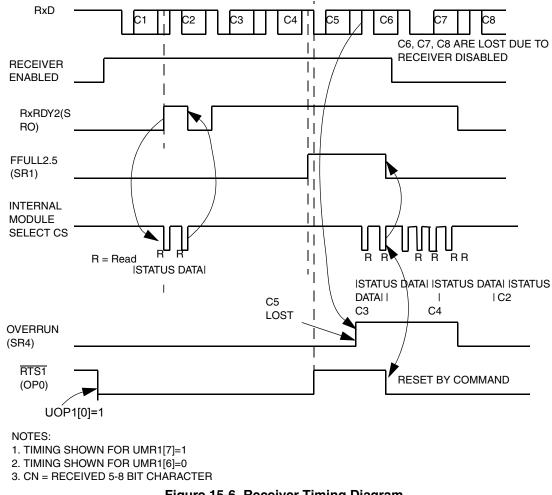
Figure 15-6. Receiver Timing Diagram
