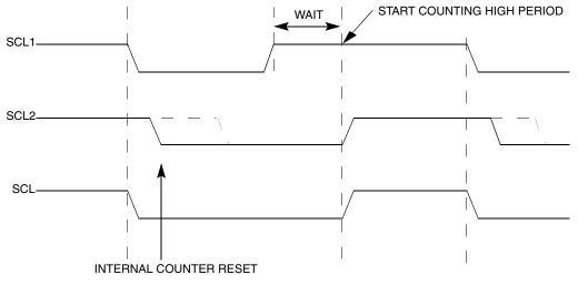
Figure 18-3. Synchronized Clock SCL
