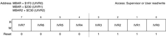
Figure 15-19. Interrupt Vector Register (UIVRn)
