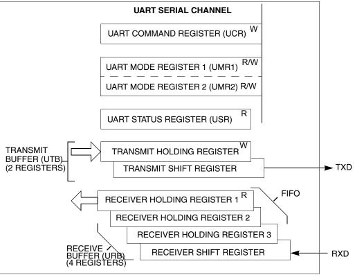
Figure 15-4. Transmitter and Receiver Functional Diagram
