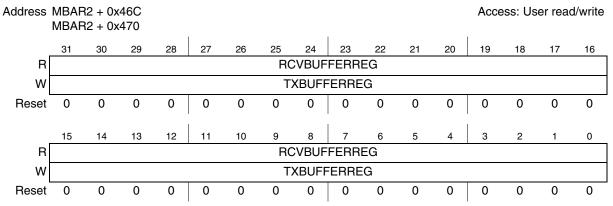
Figure 13-14. Flash Media Data Registers 1 & 2 (FLASHMEDIACMD) (Secure Digital Mode)
