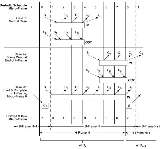
Figure 24-57. Split Transaction, Isochronous Scheduling Boundary Conditions
