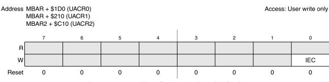
Figure 15-16. Auxiliary Control Register (UACRn)
