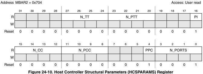
Figure 24-10. Host Controller Structural Parameters (HCSPARAMS) Re
