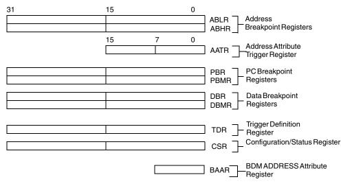
Figure 20-28. Debug Programming Mode
