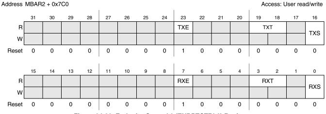
Figure 24-33. Endpoint Control 0 (ENDPTCTRL0) Register
