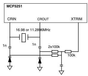
Figure 17-26. XTRIM External Circuit
