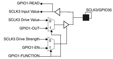
Figure 9-15. General-Purpose Pin Logic for Pin SCLK3/GPIO35
