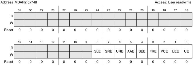
Figure 24-16. USB Interrupt Enable (USBINTR) Register
