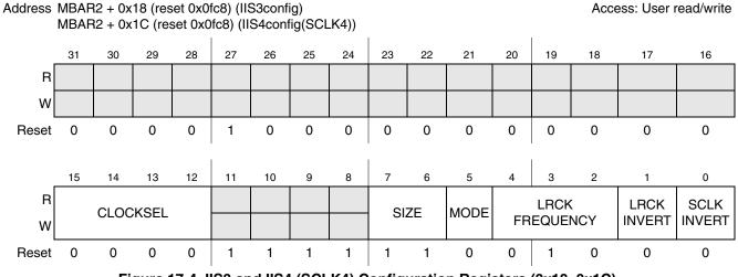
Figure 17-4. IIS3 and IIS4 (SCLK4) Configuration Registers (0x18, 0x1C)
