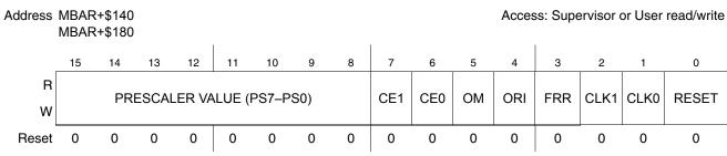
Figure 11-2. Timer Mode Register (TMRn)
