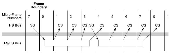
Figure 24-45. Frame Boundary Relationship between HS Bus and FS/LS Bus
