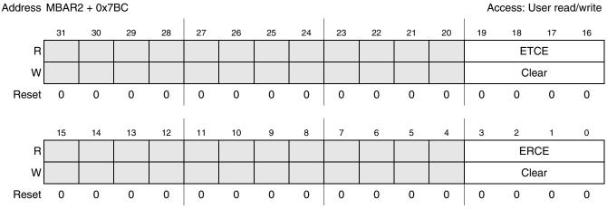
Figure 24-32. Endpoint Complete (ENDPTCOMPLETE) Register
