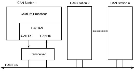
Figure 25-3. Typical CAN System
