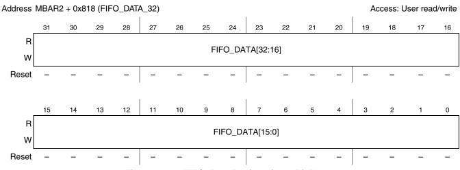
Figure 23-37. FIFO\_Data Register in 32-Bit Mode
