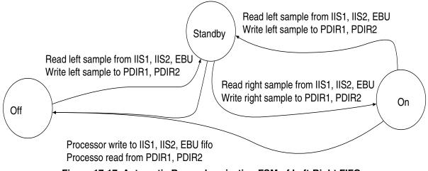
Figure 17-17. Automatic Resynchronization FSM of Left-Right FIFOs
