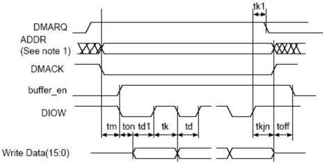
Figure 23-5. MDMA Write Timing
