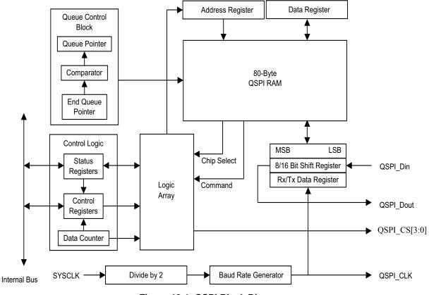
Figure 16-1. QSPI Block Diagram
