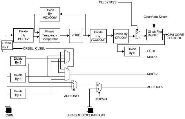
Figure 4-1. Phase-Locked Loop Module Block Diagram
