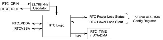
Figure 26-1. Real Time Clock Block Diagram
