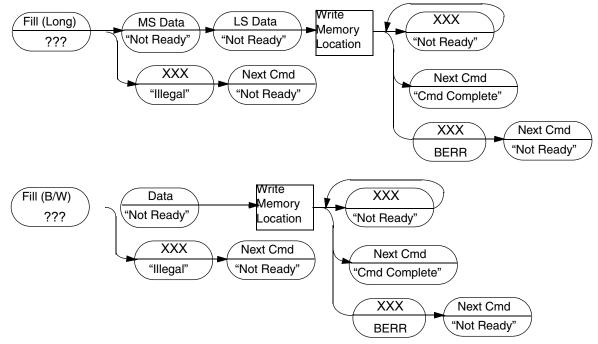
Figure 20-17. Fill Memory Block Command Sequence
