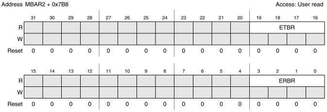
Figure 24-31. Endpoint Status (ENDPTSTATUS) Register
