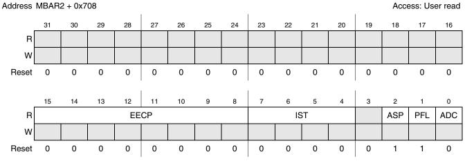
Figure 24-11. Host Control Capability Parameters (HCCPARAMS) Register
