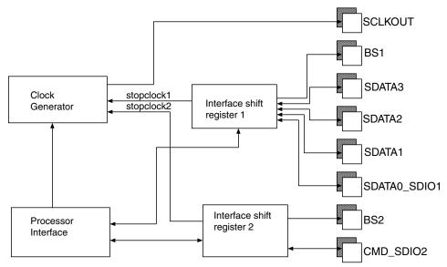
Figure 13-8. Flash Media Block Diagram
