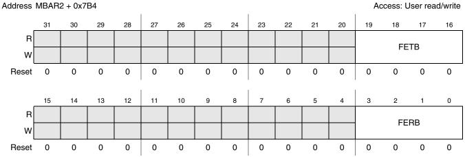
Figure 24-30. Endpoint Flush (ENDPTFLUSH) Register
