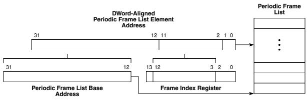
Figure 24-43. Derivation of Pointer into Frame List Array
