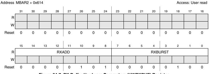
Figure 24-7. RX Buffer Hardware Parameters (HWRXBUF) Register
