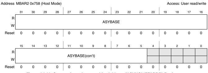
Figure 24-20. Current Asynchronous List Address (ASYNCLISTADDR) Register
