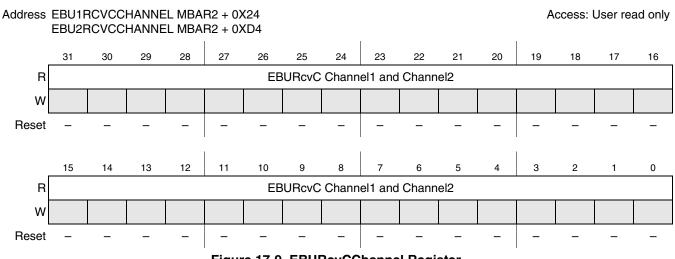
Figure 17-9. EBURcvCChannel Register
