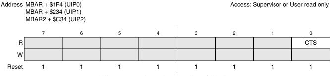
Figure 15-20. Input Port Register (UIPn)
