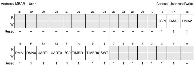
Figure 9-5. Interrupt Mask Register (IMR)
