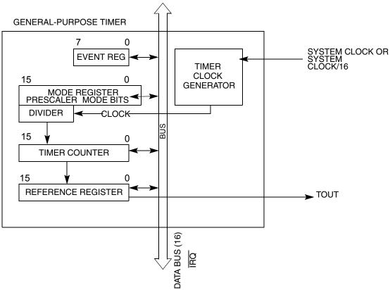
Figure 11-1. Timer Block Diagram Module Operation
