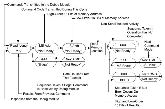
Figure 20-7. Command Sequence Diagram
