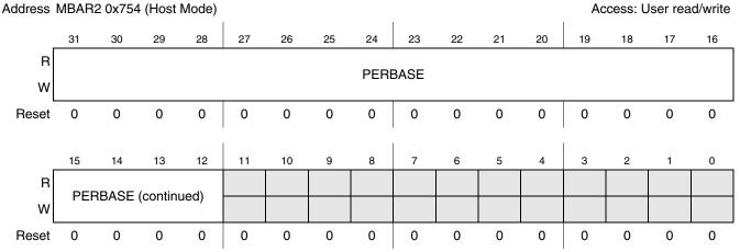
Figure 24-18. Periodic Frame List Base Address (PERIODICLISTBASE) Register
