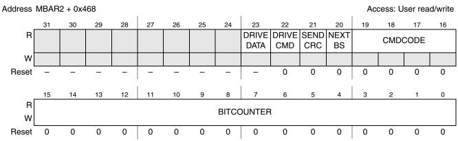
Figure 13-13. Flash Media Command Register 2 (FLASHMEDIACMD) (Secure Digital Mode)
