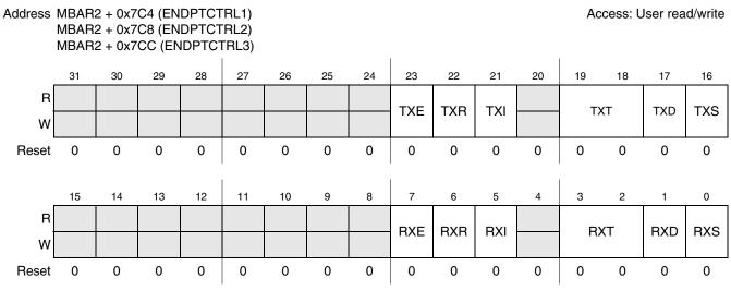
Figure 24-34. Endpoint Control 1 to 3(ENDPTCTRLn) Register
