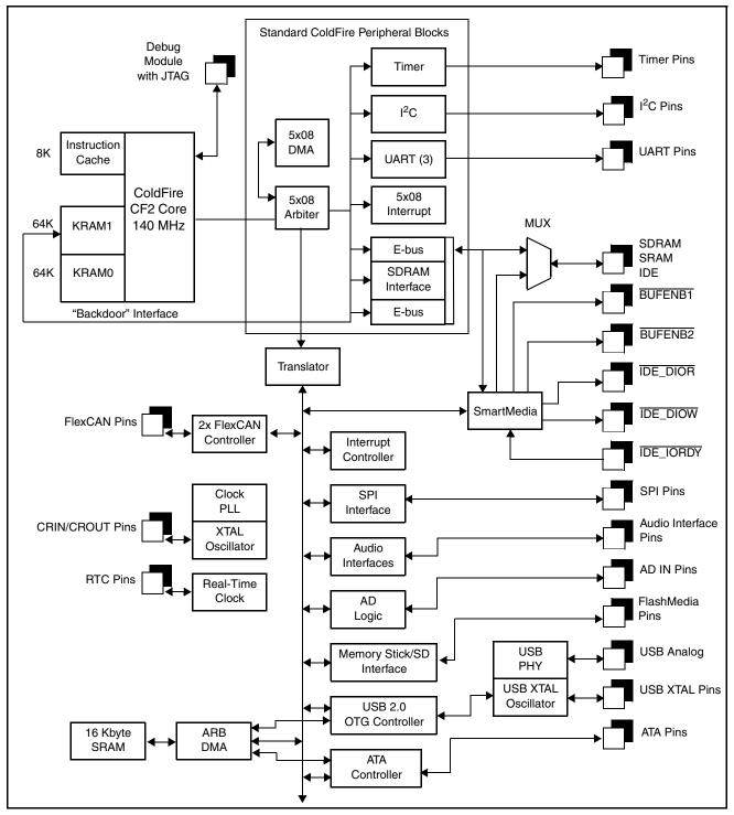
Figure 1-1. MCF5251 Block Diagram
