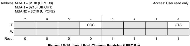
Figure 15-15. Input Port Change Register (UIPCRn)
