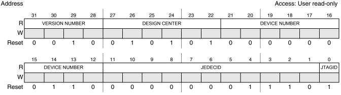
Figure 21-3. ID Code Register Command
