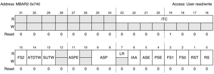
Figure 24-14. USB Command Register (USBCMD) Register
