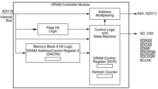
Figure 7-1. Synchronous DRAM Controller Block Diagram
