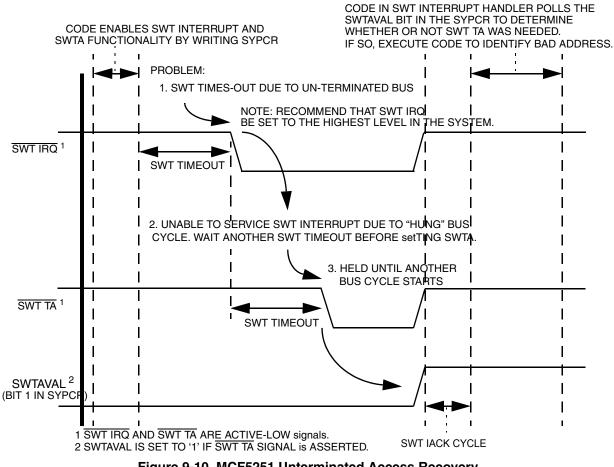
Figure 9-10. MCF5251 Unterminated Access Recovery
