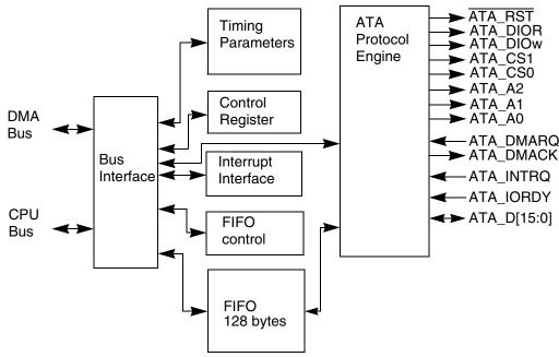
Figure 23-1. ATA Interface Block Diagram
