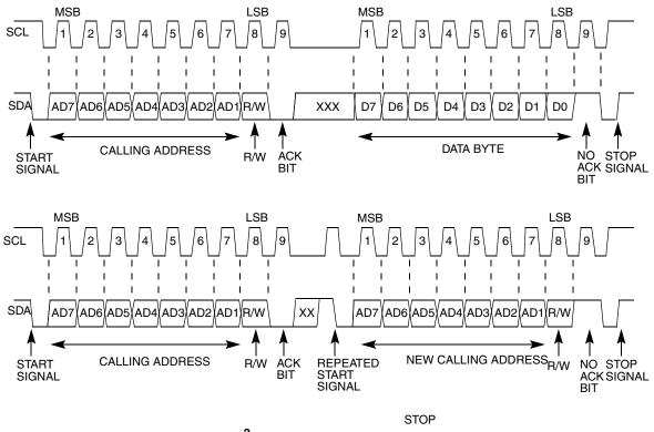
Figure 18-2. I<sup>2</sup>C Standard Communication Protocol
