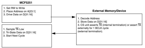
Figure 8-5. Write Cycle Flowchart
