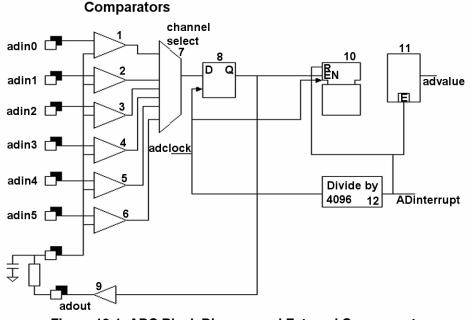
Figure 12-1. ADC Block Diagram and External Components
