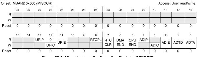
Figure 22-1. Miscellaneous Configuration Register (MISCCR)
