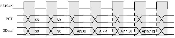
Figure 20-2. Example PST/DDATA Diagram
