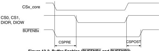
Figure 13-2. Buffer Enables (BUFENB1 and BUFENB2)
