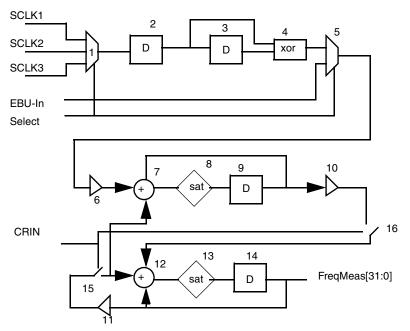
Figure 17-24. Frequency Measurement Circuit
