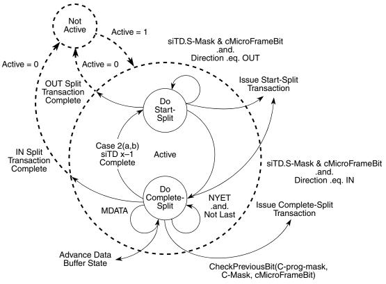
Figure 24-59. Split Transaction State Machine for Isochronous
