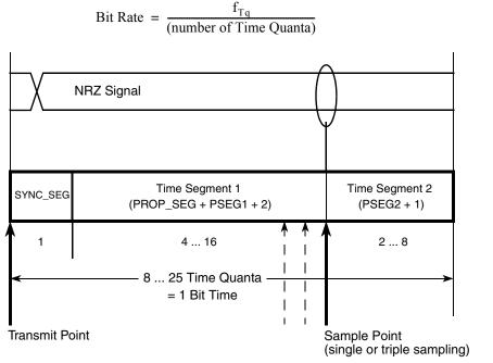
Figure 25-15. Segments within the Bit Time
