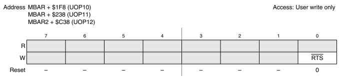
Figure 15-21. Output Port Data Registers (UOP1n)
