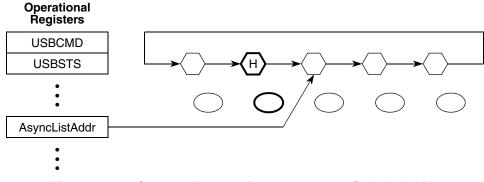
Figure 24-44. General Format of Asynchronous Schedule List
