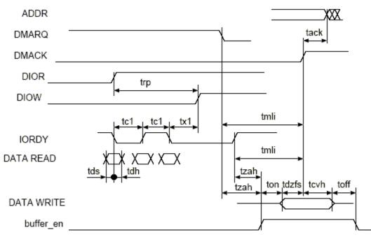
Figure 23-7. UDMA in Host Terminates Transfer
