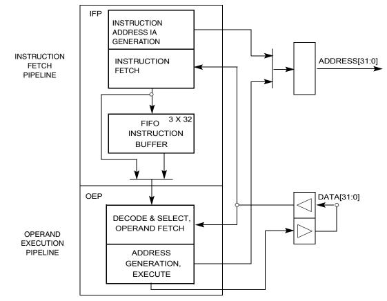
Figure 3-1 shows a block diagram of the processor pipelines of a CF2 ColdFire core.
