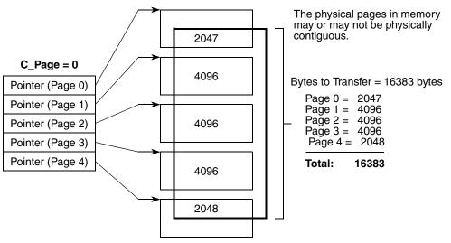
Figure 24-51. Example Mapping of qTD Buffer Pointers to Buffer Pages
