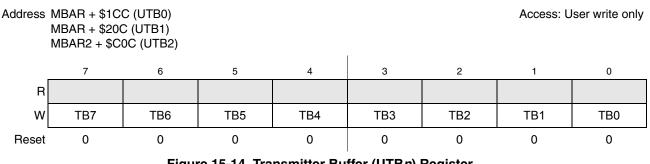
Figure 15-14. Transmitter Buffer (UTBn) Register
