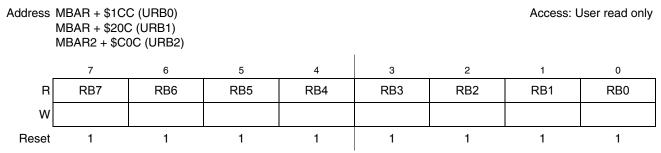
Figure 15-13. Receiver Buffer (URB*n*) Register
