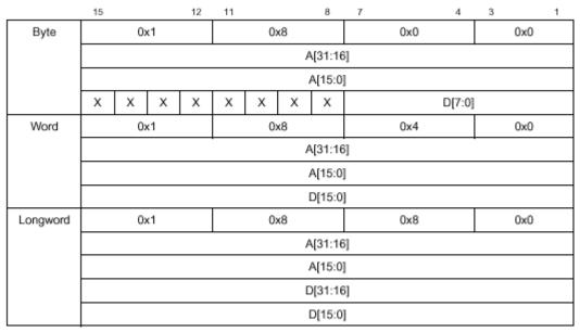
Figure 20-15. DUMP Command/Result Format
