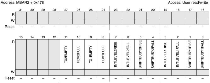
Figure 13-16. Flash Media Interrupt Register
