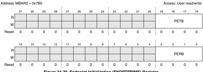
Figure 24-29. Endpoint Initialization (ENDPTPRIME) Register
