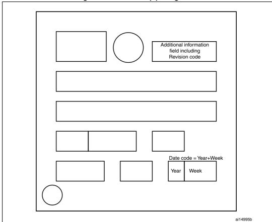
Figure 2. LFBGA100 top package view
