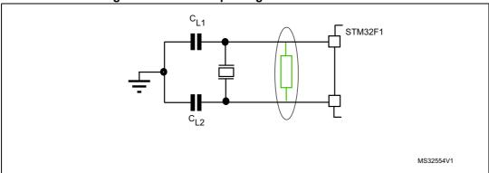
Figure 1. LSE start-up using an additional resistor
