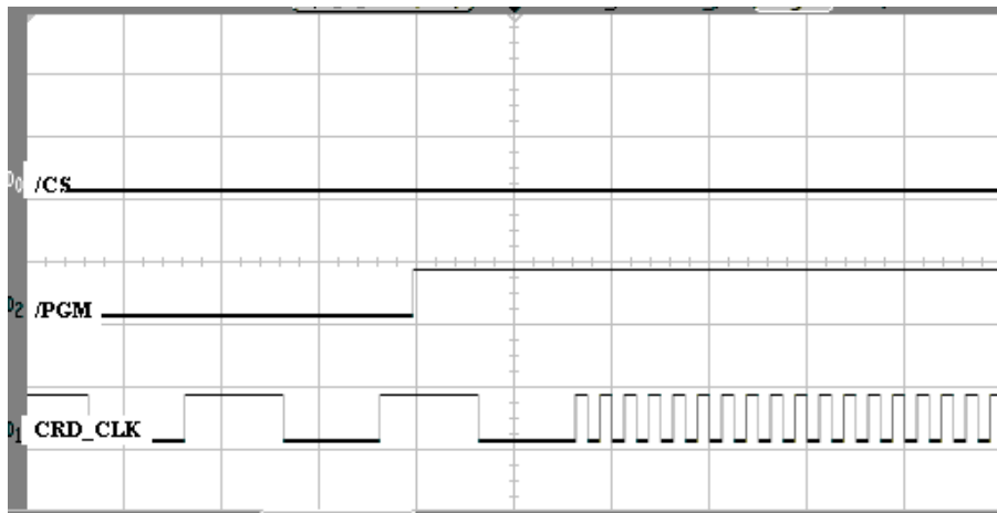
Figure 28. Clock Divider Timing Details
