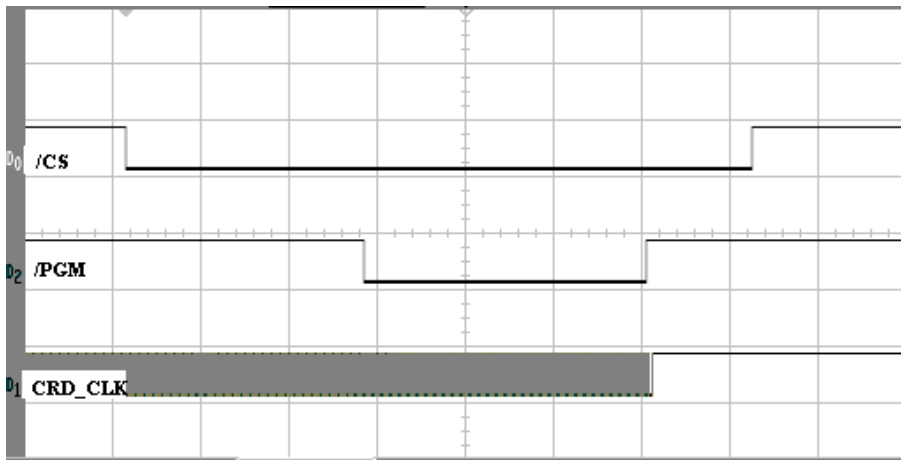
Figure 29. Clock Divider: Run to Stop High Operation
